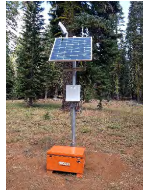
Figure 2. Base station in the Feather River basin that is hardened with upgraded hardware and communications.
