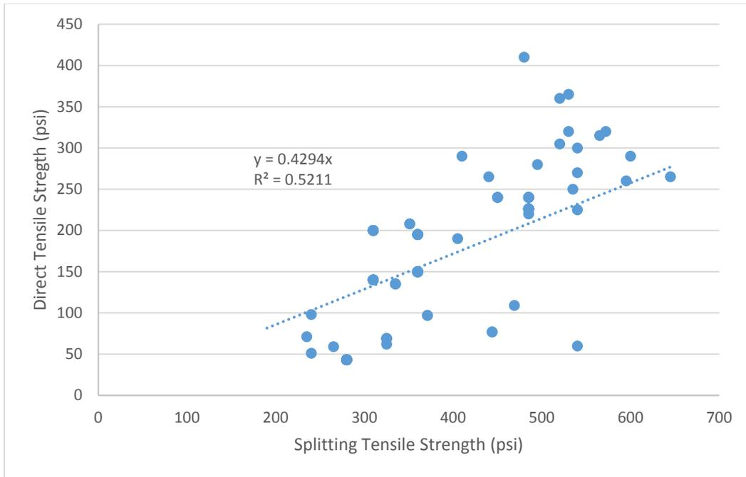
Figure 5 – All data, direct tensile versus splitting tensile strength.
