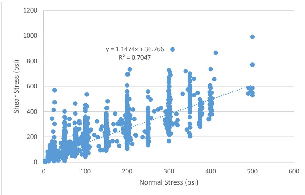
**Figure 27 – All data sliding shear strength test data with the normal stress less than or equal to 500 psi.**
