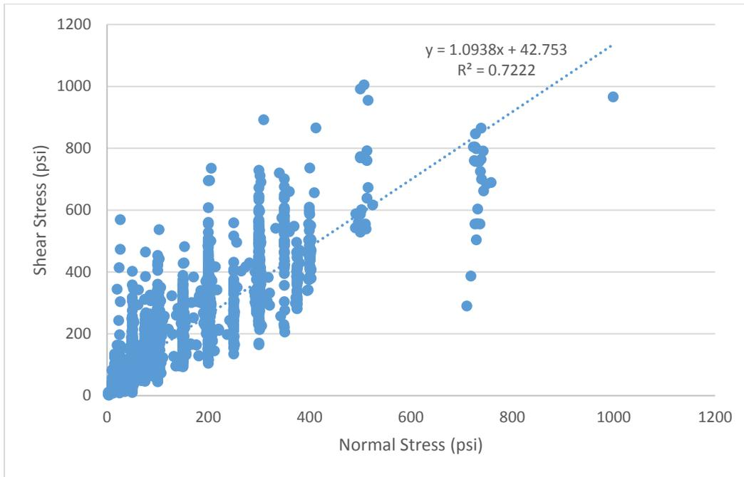
Figure 26 – All data sliding shear strength test data with the normal stress less than 1,000 psi.
