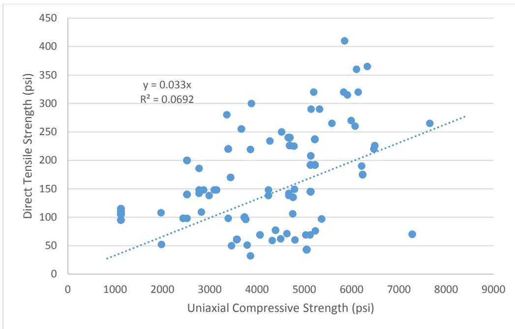
**Figure 4 – All data, direct tensile versus uniaxial compressive strength.**
