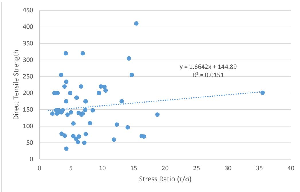
**Figure 18 - Well-constrained data break-bond direct tensile versus stress ratio. The average direct tensile strength is 158 psi.**
