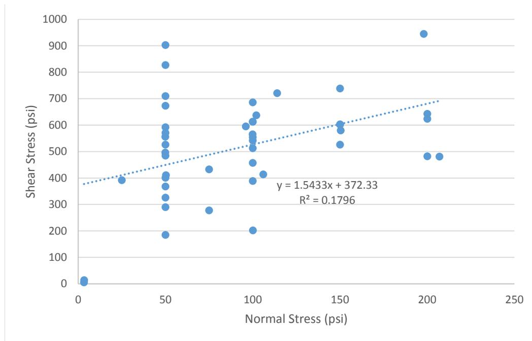
**Figure 53 - Concrete lift lines with AAR issues, break-bond shear strength data. Average UCS = 4,196 psi and average ST = 389 psi.**
