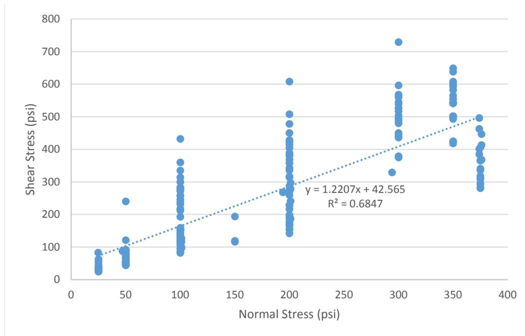
**Figure 37 - Sliding shear strength test results binned by UCS, with UCS<2,000 psi. Average UCS is 1,226 psi.**
