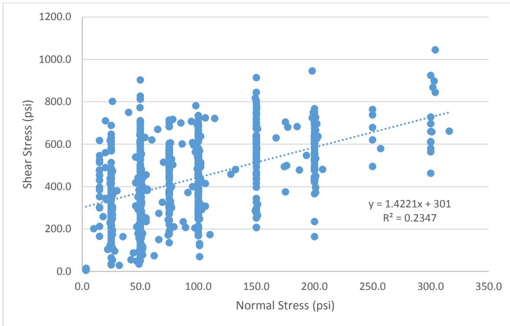
**Figure 11 – All data break-bond test data including only specimens tested at normal loads less than or equal to 316 psi.**
