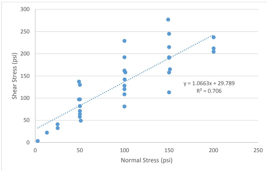
**Figure 34 - Sliding shear strength test results binned by UCS, with UCS > 6,000 psi. Average UCS = 6765 psi.**
