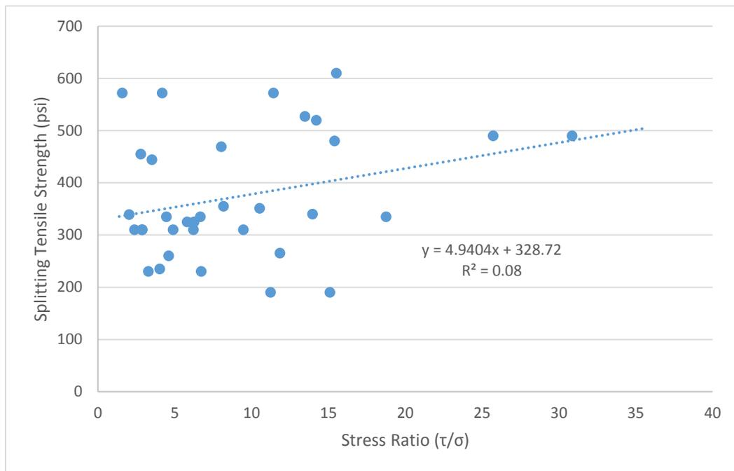
**Figure 17 - Well-constrained data break-bond splitting tensile versus stress ratio. The average splitting tensile strength is 374 psi.**
