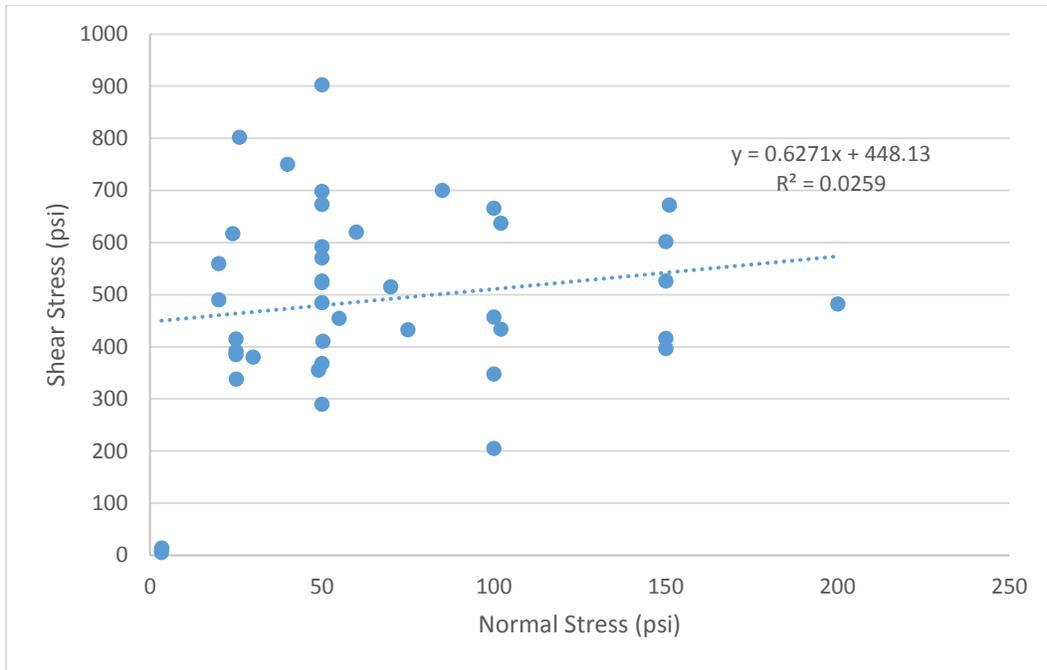
**Figure 21 – Well-constrained data break-bond strength with 4,000 psi < UCS < 6,000 psi. Average UCS = 4,715 psi.**
