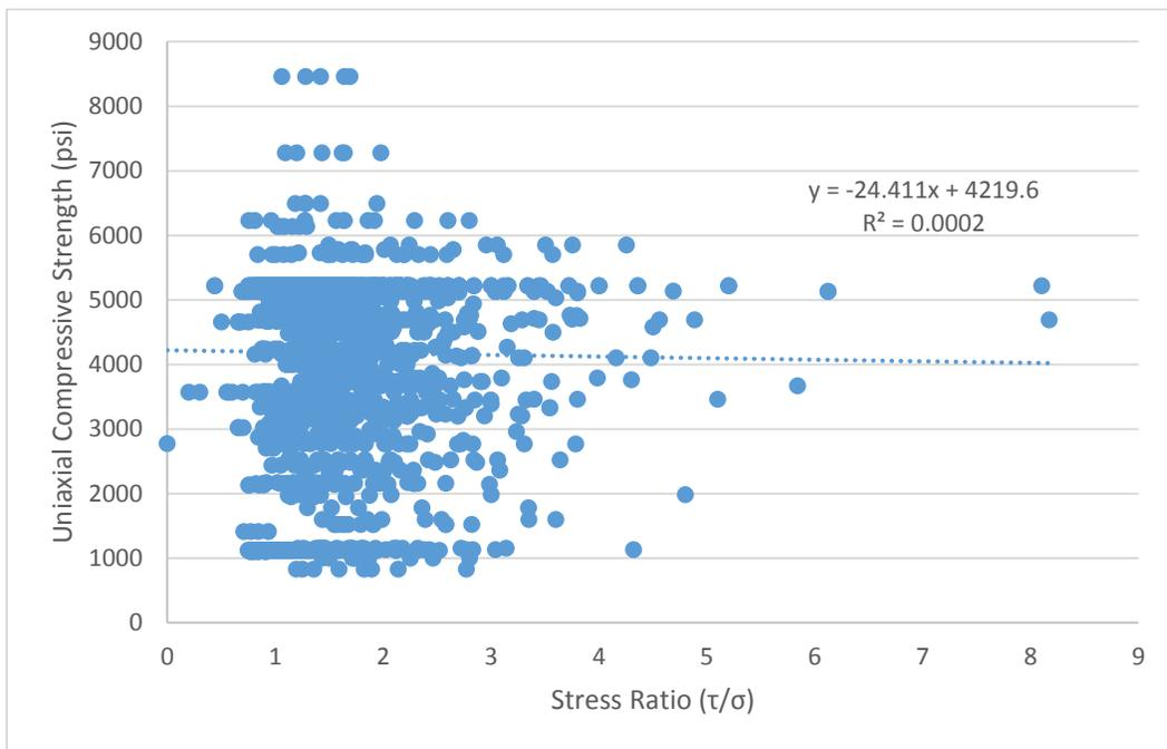
**Figure 31 – All data sliding shear strength, uniaxial compressive strength versus stress ratio.**
