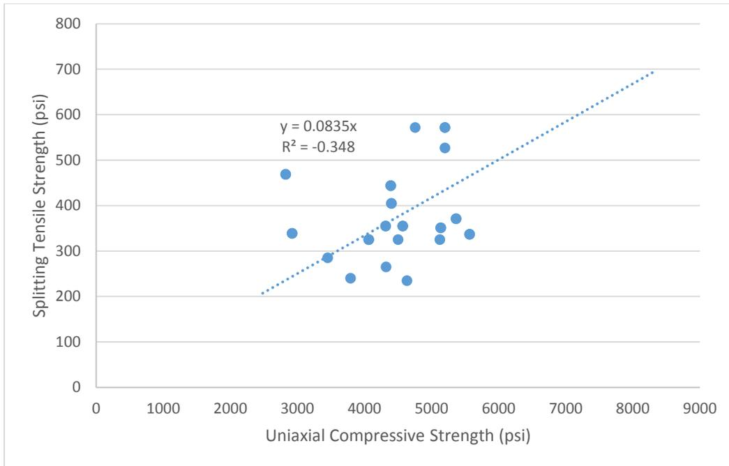
**Figure 50 - Concrete lift lines with AAR issues. Splitting tensile versus uniaxial compressive strengths. The trend line is poor and likely not valid.**
