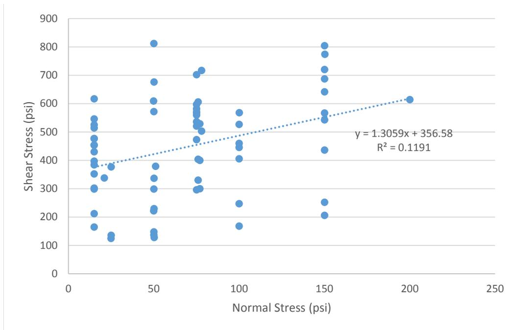
**Figure 47 - RCC lift line break-bond shear strength. Average UCS = 4,014 psi, and average ST = 485 psi.**
