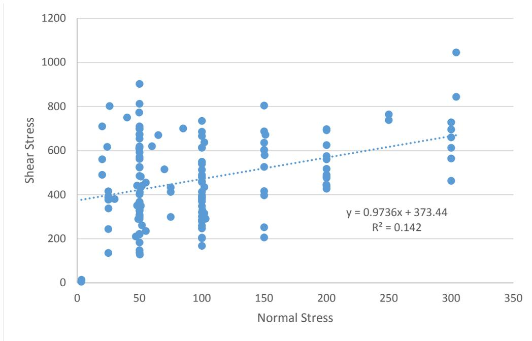
**Figure 16 – Well-constrained data break-bond test results. The average UCS = 3,397 psi, and the average ST = 374 psi.**
