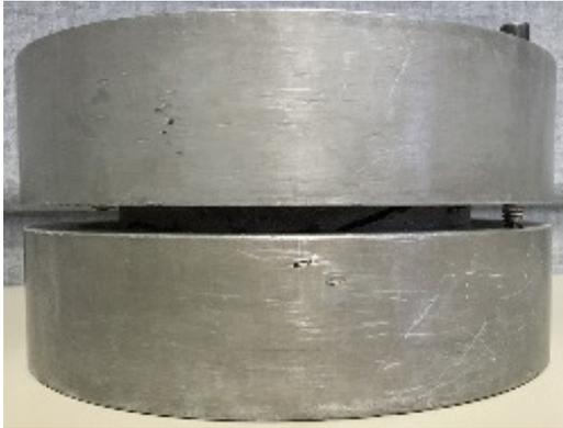
**Figure 1 - Concrete direct shear specimen encapsulated within rings. Note 0.2 inch isolated section visible between rings.**
