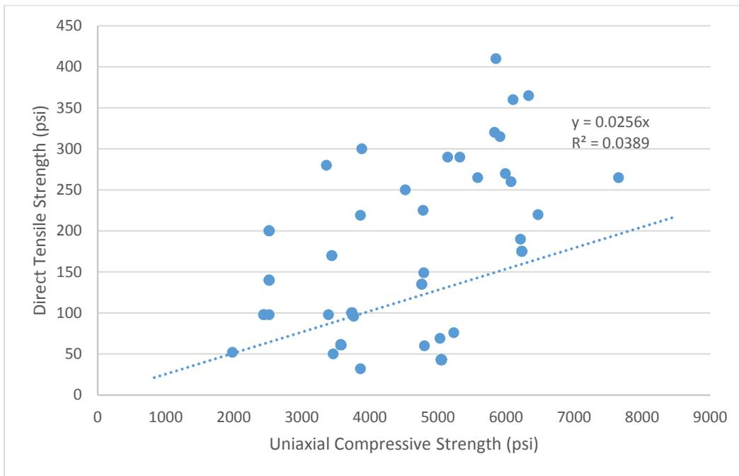
**Figure 39 - Conventional concrete lift line, direct tensile versus uniaxial compressive strength.**
