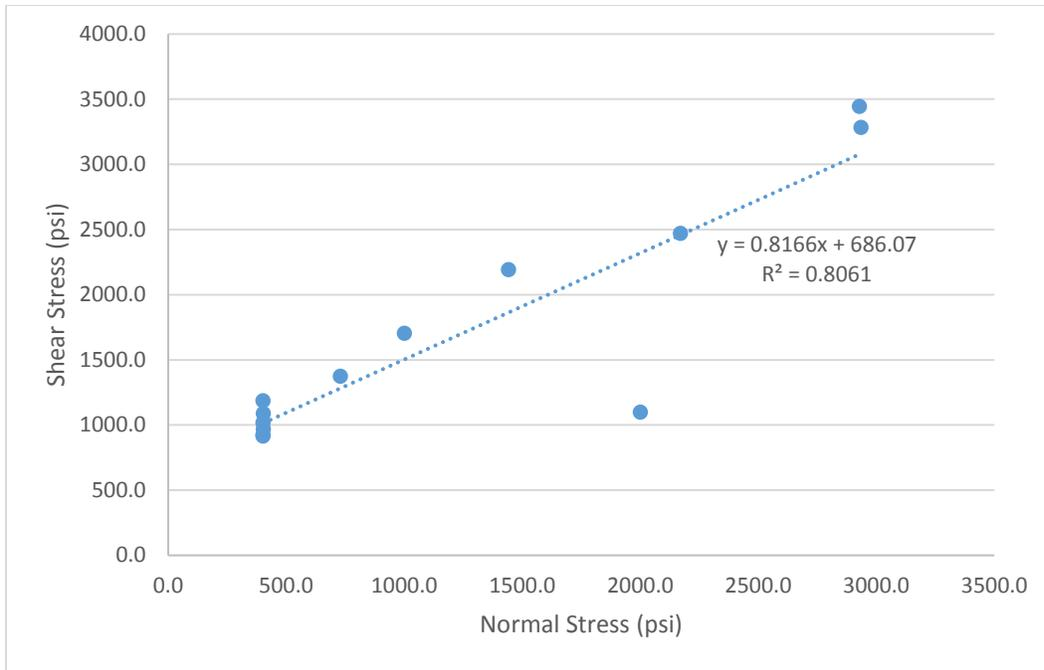
**Figure 10 – All data break-bond test results including only specimens tested at normal loads greater than 400 psi.**
