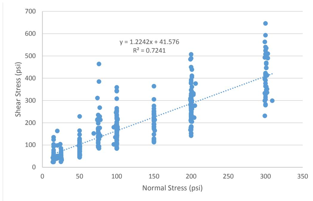
**Figure 49 - RCC lift line sliding shear strength.**
