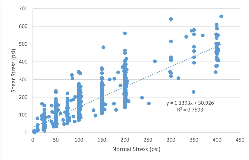
**Figure 35 - Sliding shear strength test results binned by UCS, with 4,000 psi<UCS<6,000 psi. Average UCS = 5,000 psi.**
