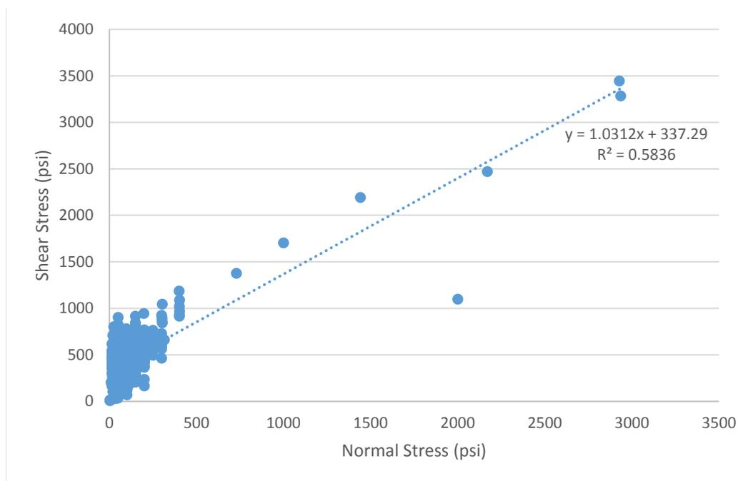
**Figure 9 – All data break-bond test results. The average UCS = 4,239 psi, and the average ST = 359 psi.**
