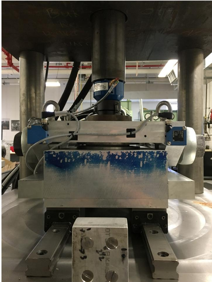
**Figure 2 - Direct shear specimen in testing machine. Normal actuator used to apply constant normal stress. Top shear box remains stationary while bottom shear box moves towards camera at a constant rate. Note 0.2 inch isolated section between shear boxes.**
