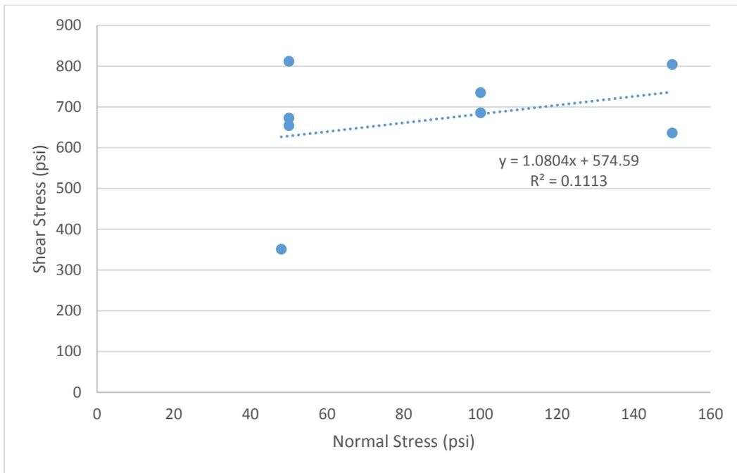
**Figure 20 – Well-constrained data break-bond strength with UCS>6,000 psi. Average UCS = 6,760 psi.**
