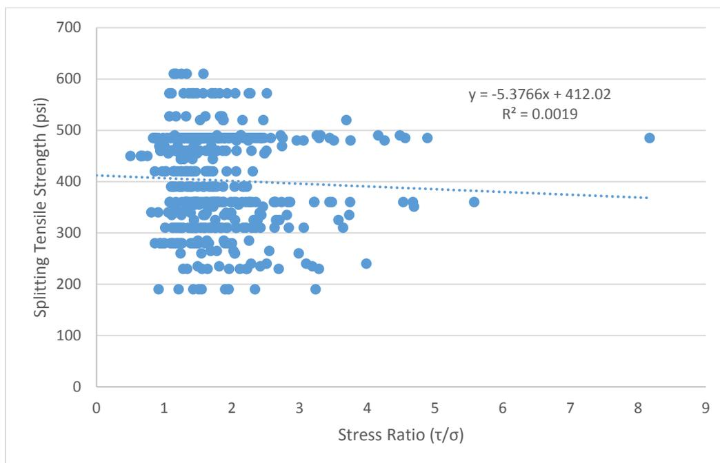
Figure 29 – All data sliding shear strength, splitting tensile strength versus stress ratio.
