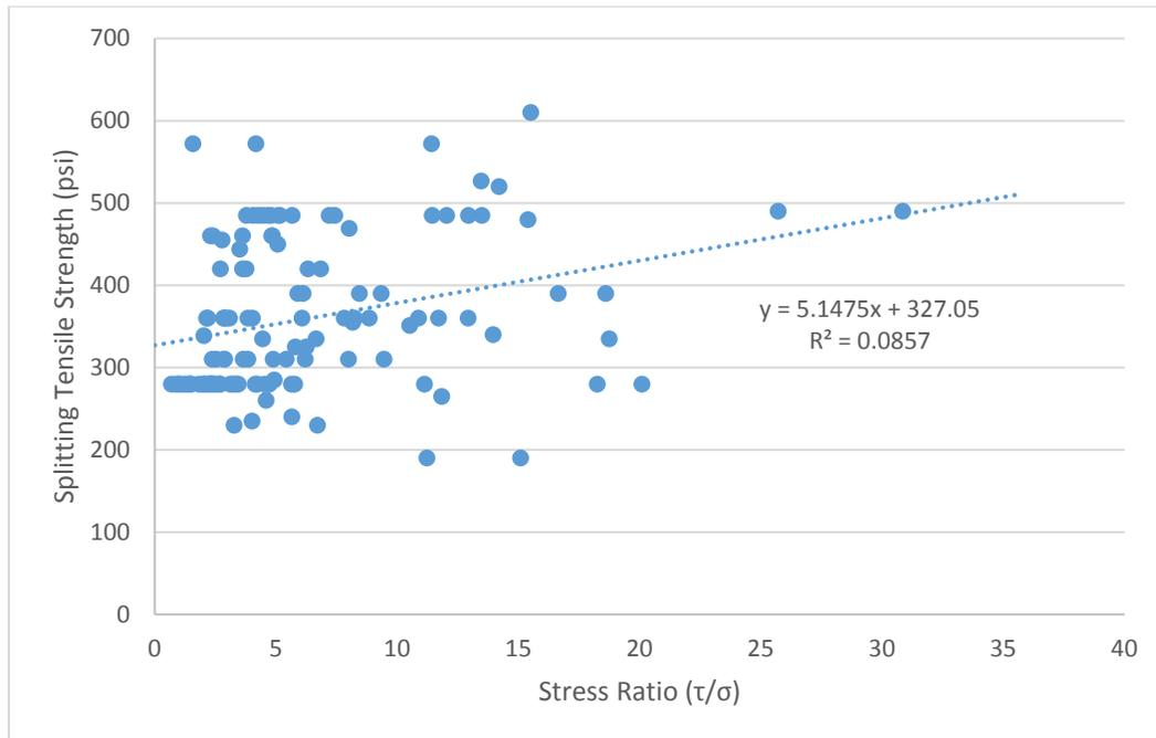
**Figure 12 – All data break-bond splitting tensile versus stress ratio. The average splitting tensile strength is 359 psi.**
