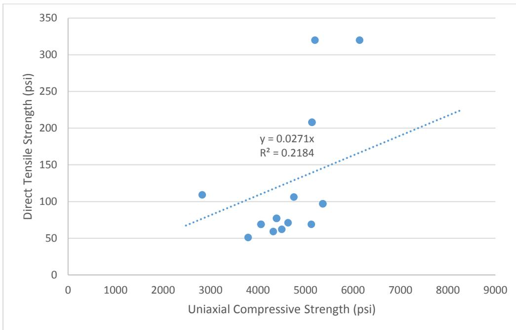
**Figure 51 - Concrete lift lines with AAR issues. Direct tensile versus uniaxial compressive strength.**
