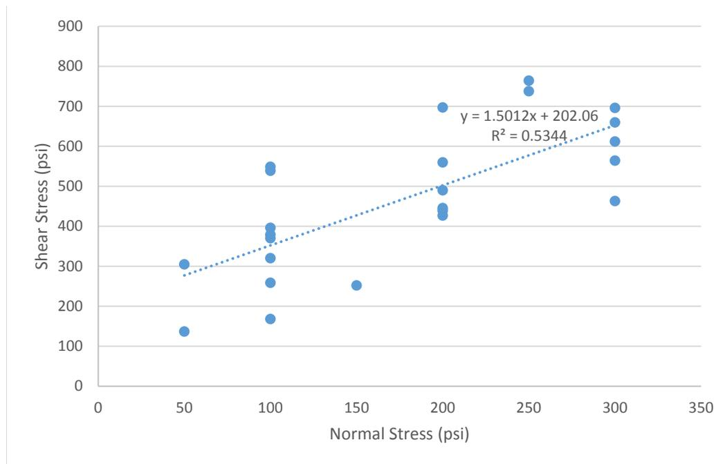
**Figure 23- Well-constrained data break-bond strength with UCS<2,000 psi. Average UCS = 1,328 psi.**
