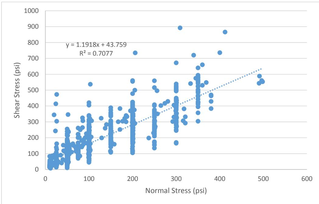
**Figure 46 - Conventional concrete lift line sliding shear strength with normal stress less than 500 psi.**
