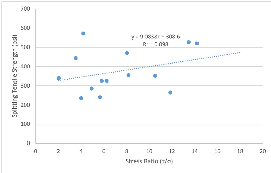
**Figure 54 - Concrete lift lines with AAR issues break-bond. Splitting tensile strength versus stress ratio.**
