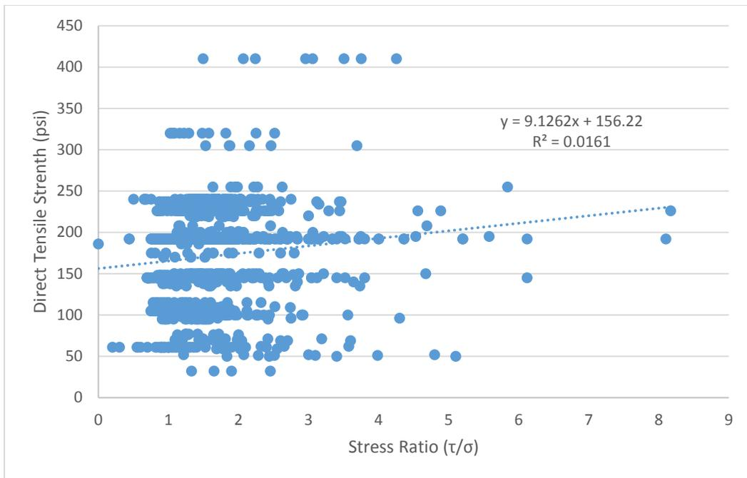
**Figure 30 – All data sliding shear strength, direct tensile strength versus stress ratio.**
