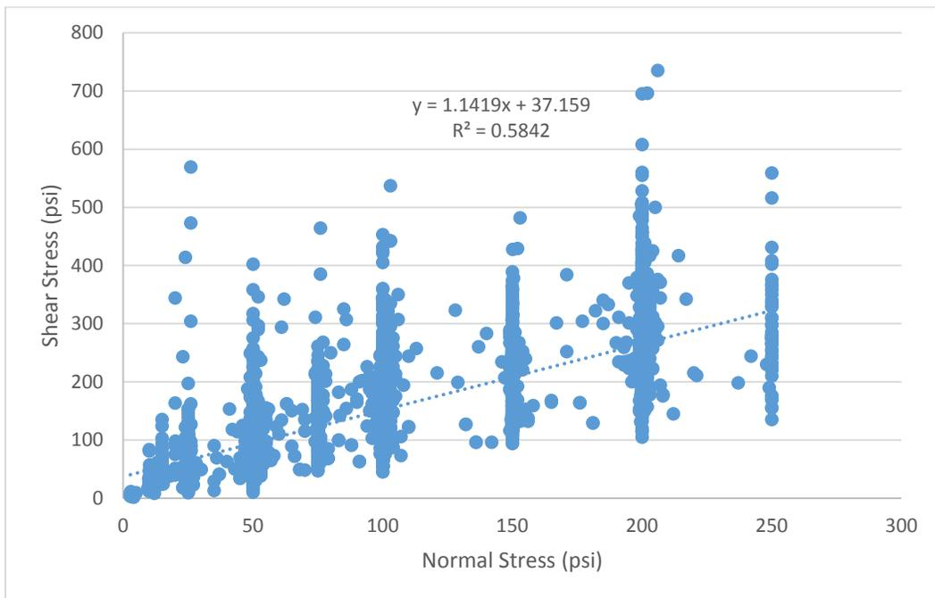
**Figure 28 – All data sliding shear strength test data with the normal stress less than or equal to 250 psi.**
