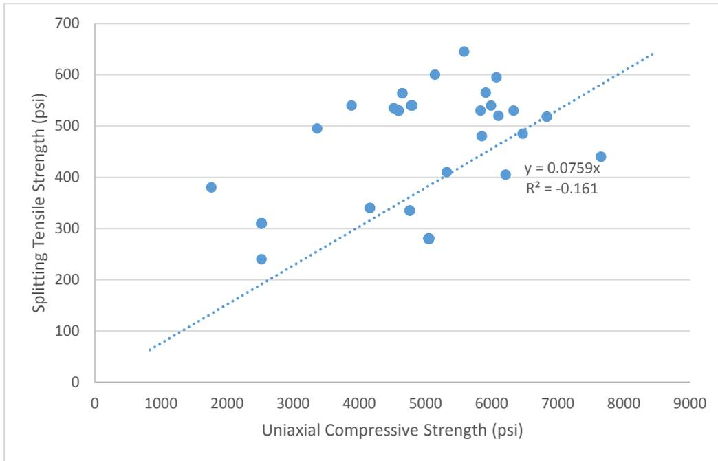
**Figure 38 - Conventional concrete lift line, splitting tensile versus uniaxial compressive strength.**
