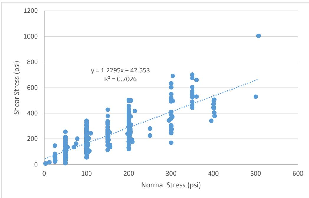
**Figure 36 - Sliding shear strength test results binned by UCS, with 2,000 psi<UCS<4,000 psi. Average UCS is 3,140 psi.**
