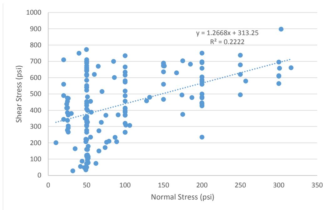
**Figure 41 – Conventional concrete lift line break-bond shear strength. Average UCS = 4188 psi, and average ST = 382 psi.**
