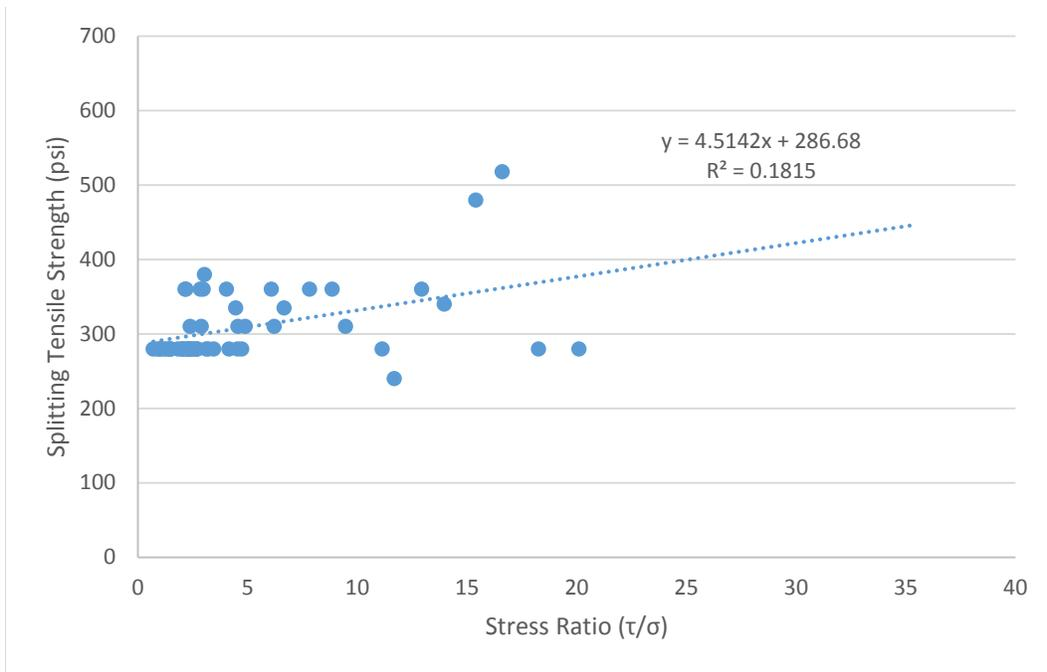
Figure 42 - Conventional concrete lift line break-bond data showing splitting tensile strength versus stress ratio.
