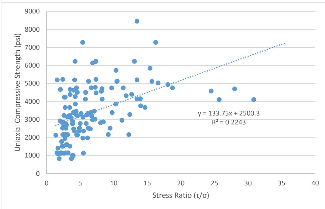
**Figure 19 - Well-constrained data break-bond uniaxial compressive strength versus stress ratio. The average uniaxial compressive strength is 3,397 psi.**
