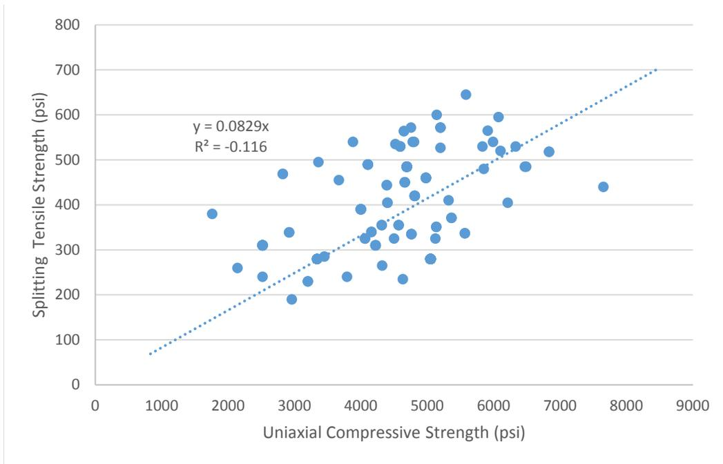
**Figure 3 – All data, splitting tensile versus uniaxial compressive strength.**
