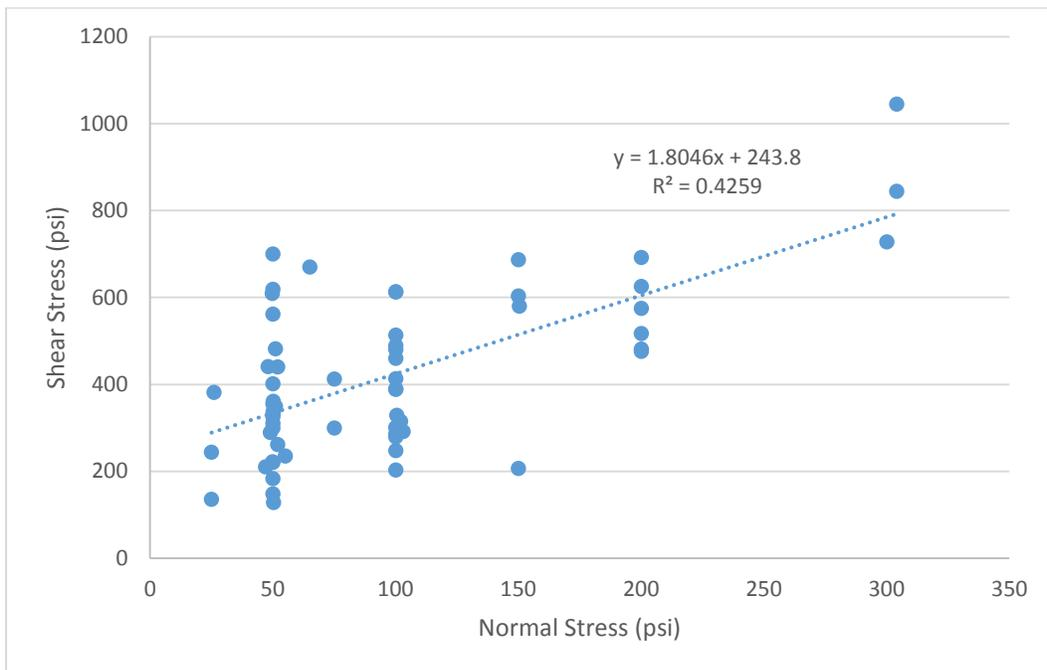
**Figure 22 – Well-constrained data break-bond strength with 2,000 < UCS < 4,000 psi. Average UCS = 2,893 psi.**
