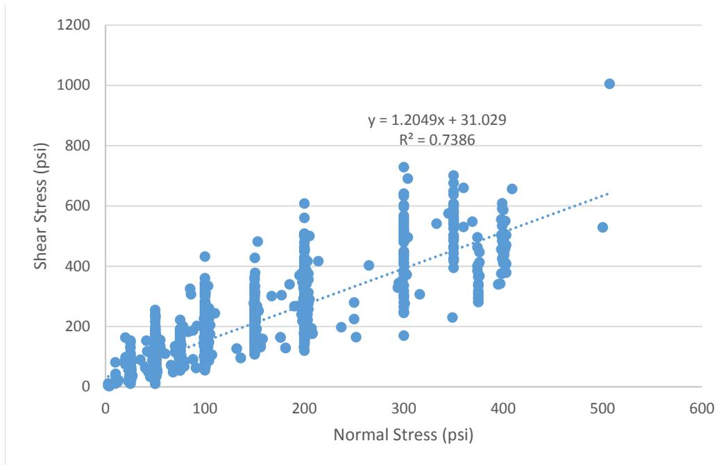
**Figure 33 - Sliding shear strength test results only for specimens that had accompanying UCS values. Average UCS = 4,180 psi.**
