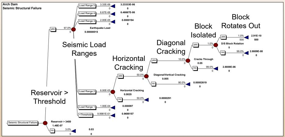
Note: Only **one** reservoir range is critical in this example. Analyses may indicate diagonal cracking occurs first (adjust event tree), Temperature ranges not evaluated.
