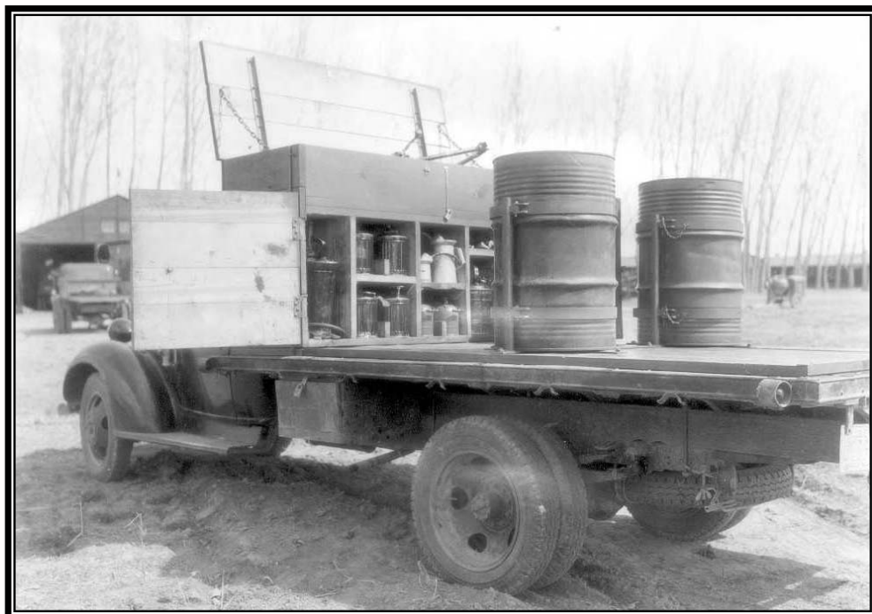
Camp BR-72: Shoshone Project, fuel and service truck with compartments, May 1, 1941 (Box 2, Entry 31, RG 115, National Archives, Denver).
