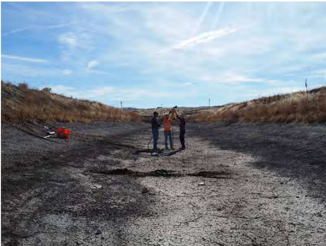
Figure 26. Installing temperature rods in the Truckee Canal for measuring diffuse seepage using the heat as a tracer approach.
