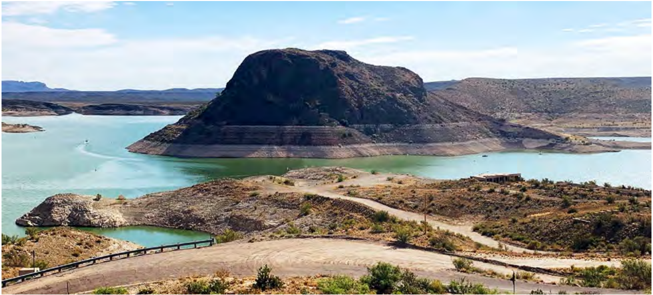
Figure 2. Elephant Butte Reservoir in New Mexico at 11 percent of water storage capacity. The white bathtub rings on the bank mark previous higher water levels.
