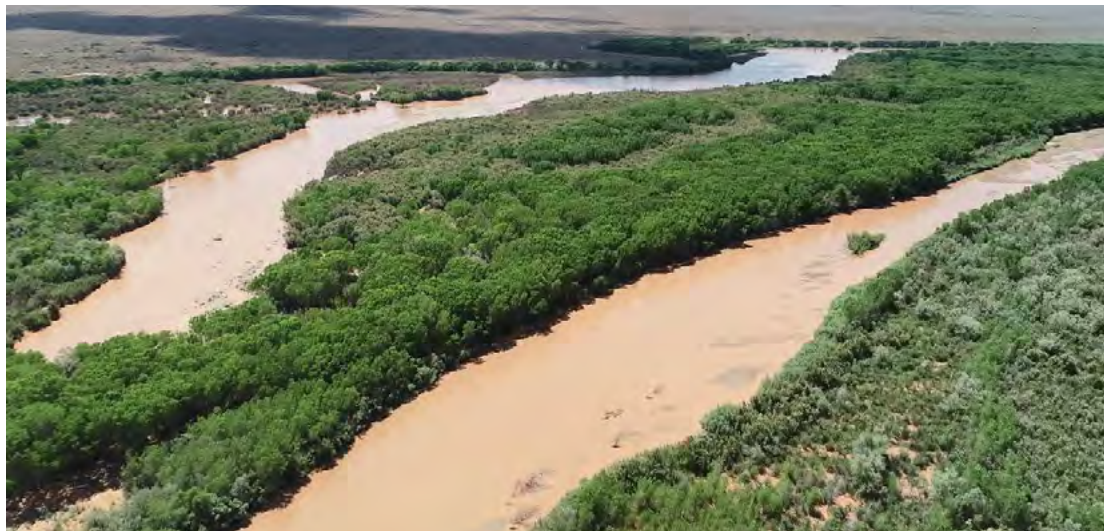
Figure 29. Channel realignment to alleviate perching upstream of Elephant Butte Reservoir in New Mexico.
