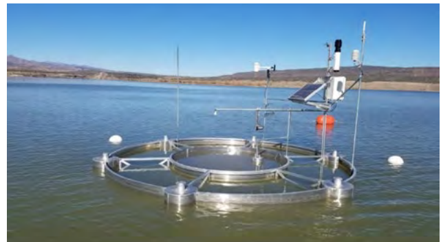
Figure 23. A Collision Floating Evaporation Pan deployed at Cochiti Lake in central New Mexico.
