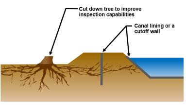
Figure 21. Acceptable methods to cutoff root systems.
