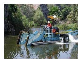
Figure 24. Combination hydrocutter and harvester.
