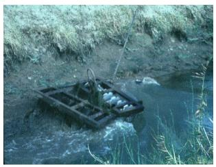
Figure 25. Tandem disc cultivator on a drag chain in an irrigation ditch used to disrupt rooted weeds.
