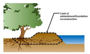
Figure 20. Example of embankment/foundation reconstruction limits.
