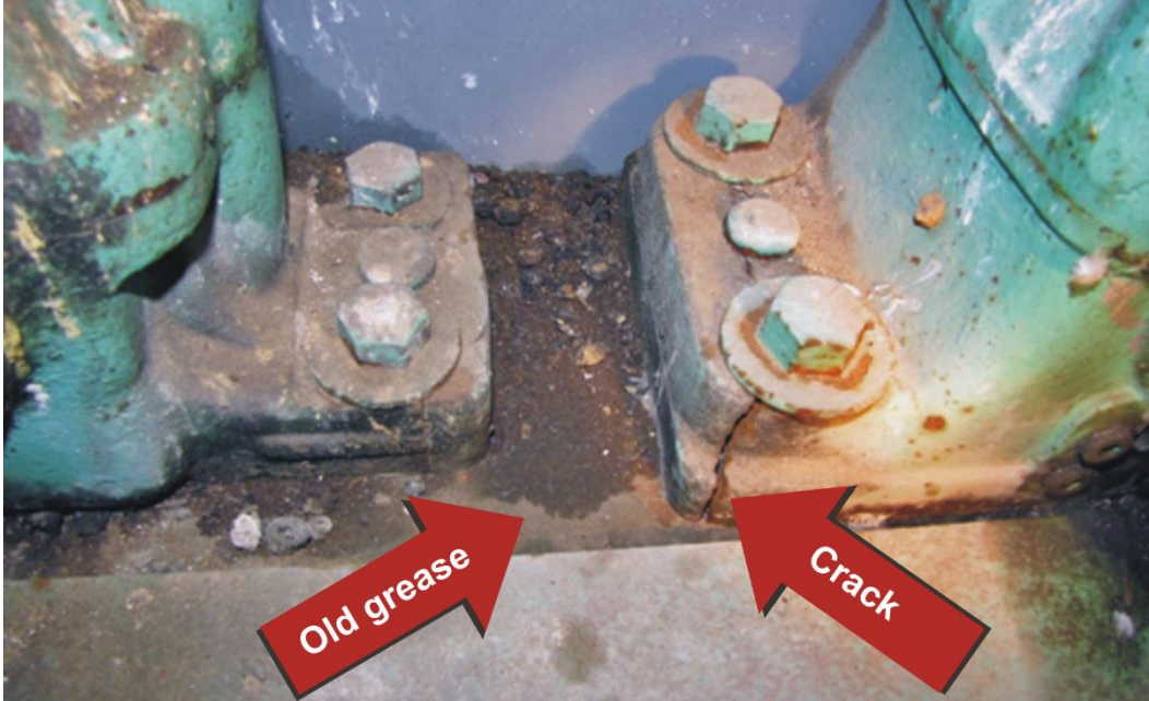
Figure 6. Hardened lubricant led to misalignment of gears, causing the pillow block to move downstream and crack.
