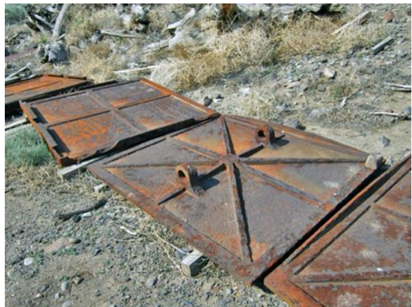
Figure 3. If there is too much corrosion, your gates won't hold water.
