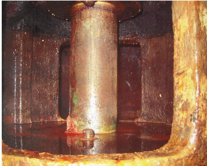
Figure 19. A flooded stem packing will cause corrosion and damage the packing.
