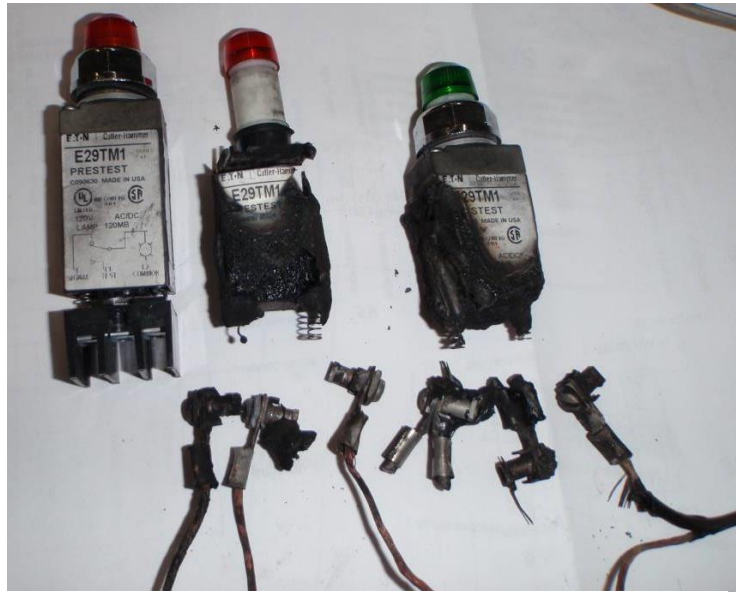
Figure 27. Rear view of indicating light terminal connections (fault initiated on lugs connected to center red light terminal). Fault caused by a loose screw connection and a malfunctioning circuit breaker.
