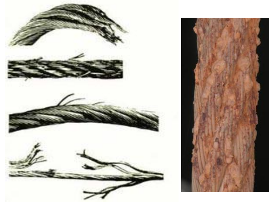
Figure 9: Common damage on wire ropes.
