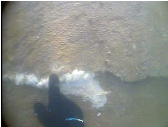
Figure 23. Chemical grout product A with 120 °F pre-mixed injection water.
