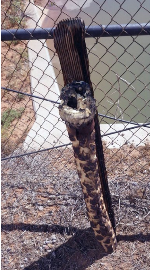
Figure 45. O&M personnel burned debris collected from the canal next to a test station and melted it, so the test station had to be replaced.
