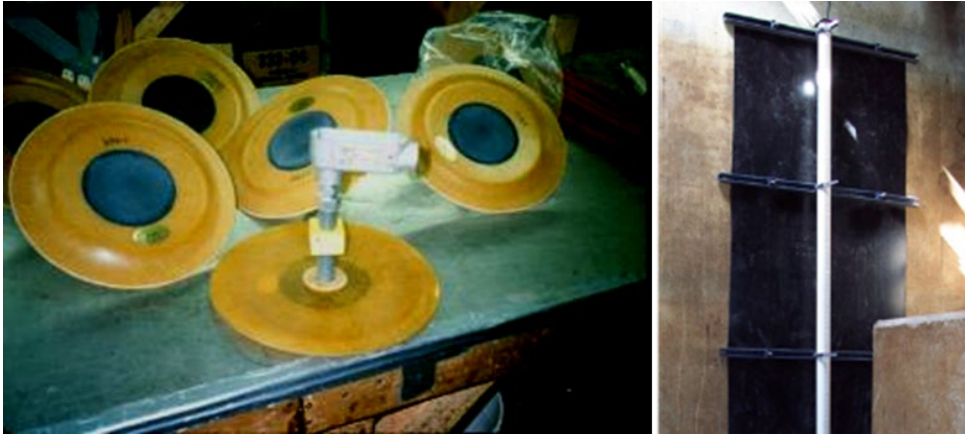
Figure 33. Impressed current anodes for submerged service. The photo on the left is a flush mounted MMO disk anode and the photo on the right a platinum/niobium wire anode in a slotted tube.
