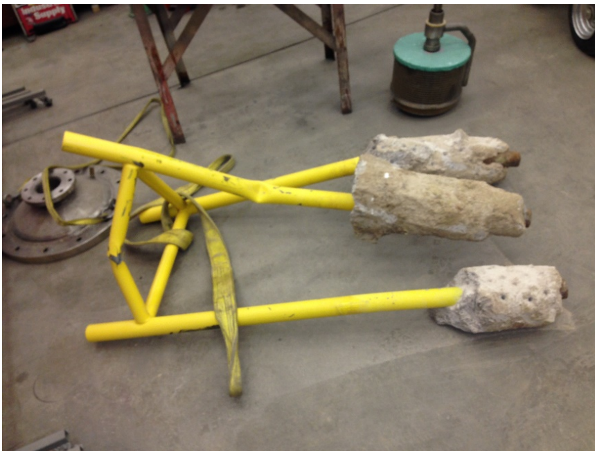
Figure 46. Test station damaged during the removal of vegetation.
