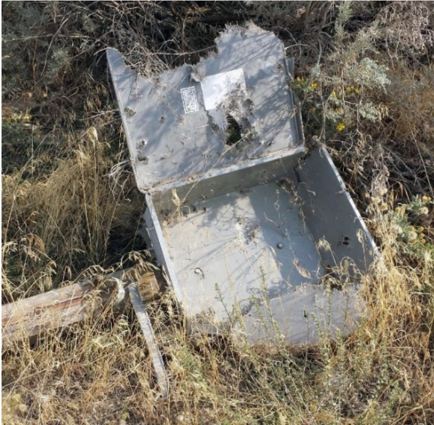
Figure 44. Vandalism of junction box—shot, knocked down, and copper cable removed for salvage.
