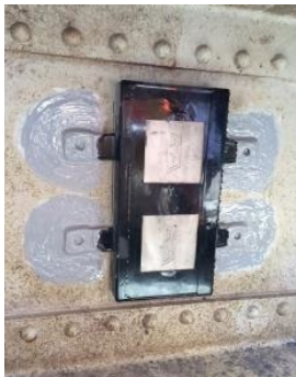
Figure 30. Magnesium galvanic hull mount anode with plastisol coating for submerged use.
