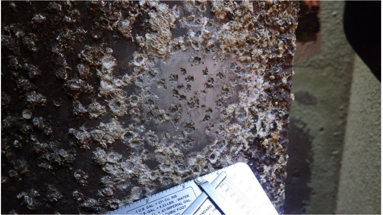
Figure 8. Pitting corrosion on an aluminum gate due to environmental changes from invasive mussels.
