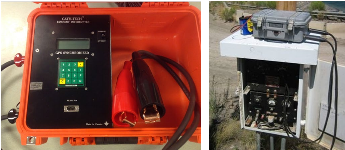
Figure 52. Current interrupter: used to automatically switch the current on and off at set intervals. Used to measure the polarized or “instant-off” potential.
