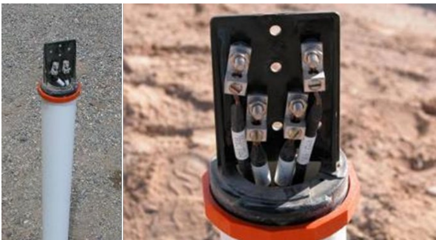
Figure 34. Big Fink style corrosion monitoring test station (left) and isolation test station (right).
