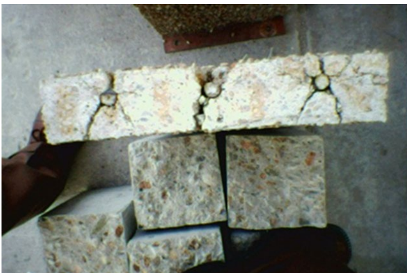
Figure 11. Cracking of the concrete occurs parallel to the corroding steel reinforcement.
