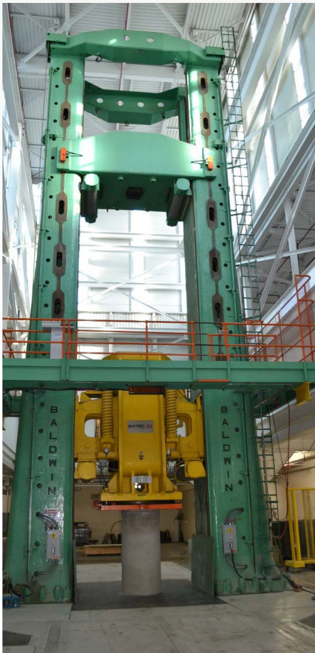
Reclamation's iconic 5,000,000-Pound Testing Machine.
