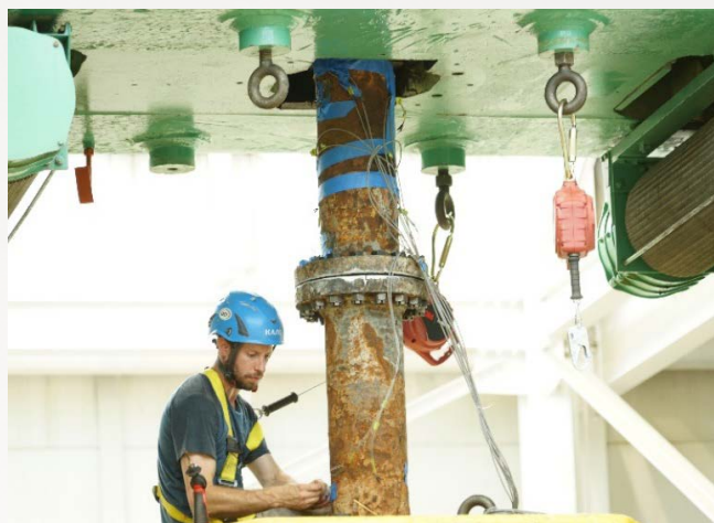
Nickel adding strain gages to gate stems in the testing machine.
