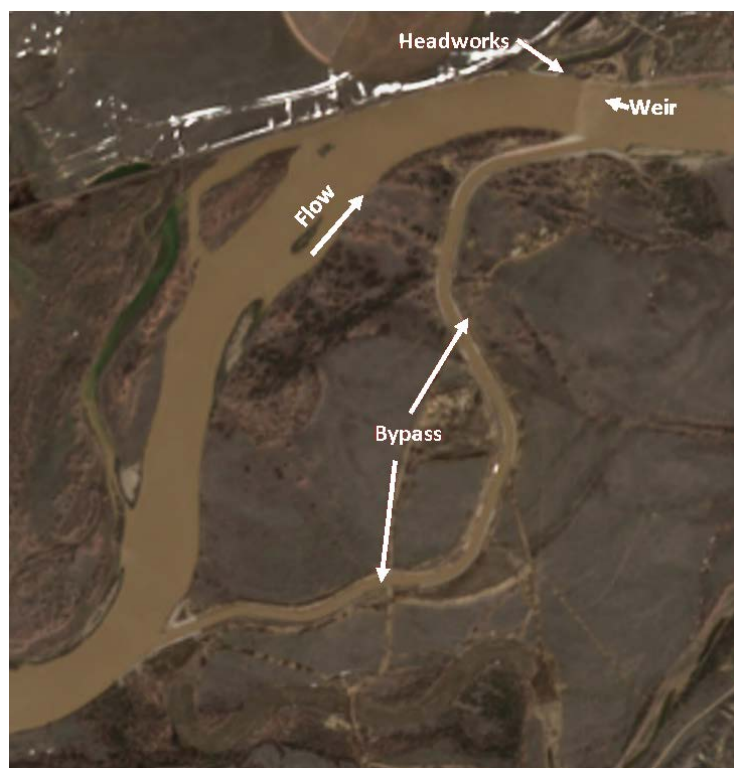
Aerial view of the Lower Yellowstone Project showing the fish bypass, diversion weir, and headworks.
