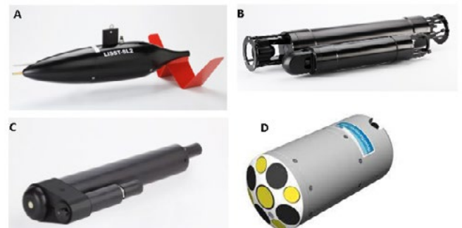
Surrogate sediment sampling devices. A: LISST-SL2 and B: LISST-200X: laser devices for particle size and volumetric sediment concentration. C: LISST-AOBS: acoustic and optical device for suspended sediment concentrations. D: SonTek M9: acoustic Doppler current profiler for suspended sediment concentrations. (credit Sequoia Scientific (A-C), SonTex/Xylem (D))
