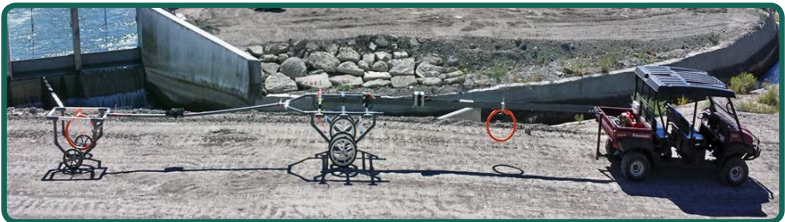
Two non-magnetic carts used for geophysical profiling with an EM34 system along South Canal near Montrose, Colorado. Here, a tandem cart configuration is required to mount the EM34 transmitter and receiver coils (orange hoops) at a minimum separation of 30 feet. Among other factors, the larger separation of the EM34 system coils results in a greater depth of investigation, compared to smaller and more compact EM systems.
