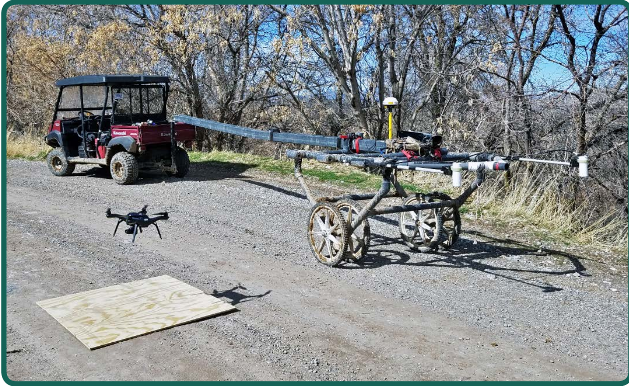
An unmanned aerial vehicle landing after collecting data along the Strawberry Highline Canal near Provo, Utah and a non-magnetic cart used for geophysical profiling along canal embankments.
