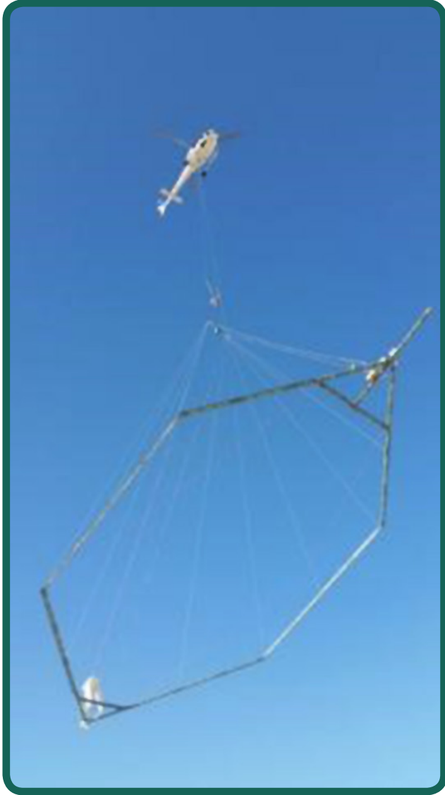
The airborne time-domain electromagnetic survey, during Yuma flights in early September 2016. (Photo courtesy of Jared Abraham - Aqua Geo Frameworks)
