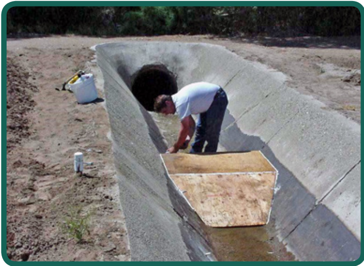
Temporary plywood structures can demonstrate how well the structure measures water and can help determine where permanent structures should be placed.
