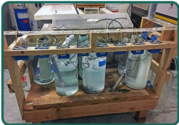
Our cathodic disbondment test to test coatings on a pipe in conjunction with cathodic protection.
