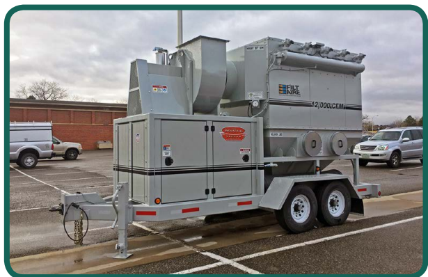
Our newly acquired dust collector that will enable us to go out in the field and complete small coatings jobs.
