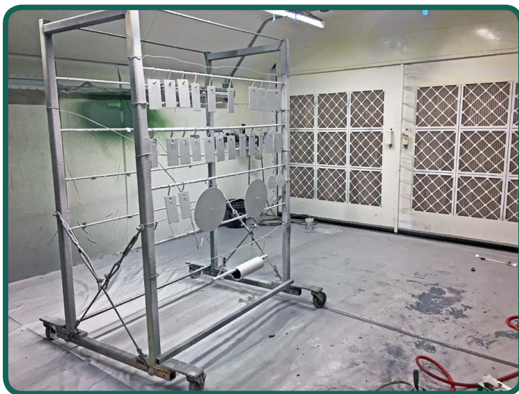
Our new, state-of-the-art paint booth where we spray the coatings that we test.
