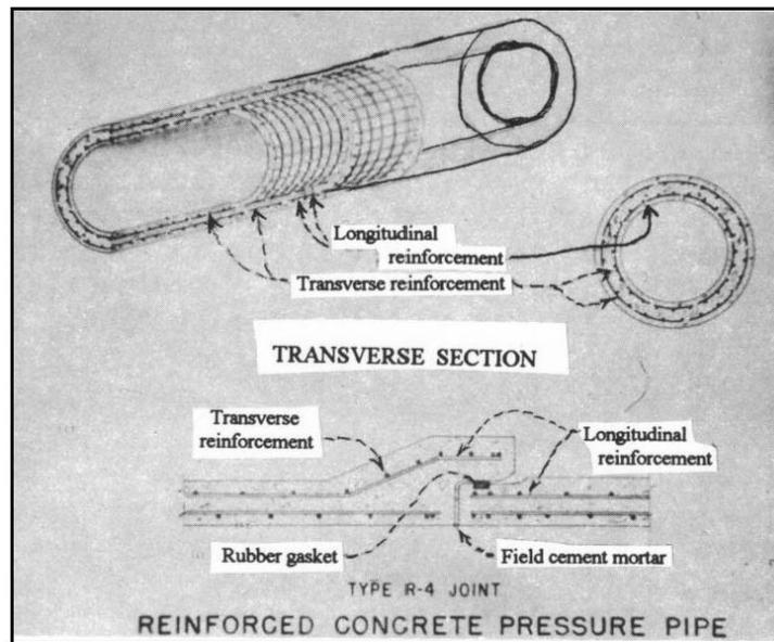
Figure 1.—Reinforced concrete pressure pipe.
