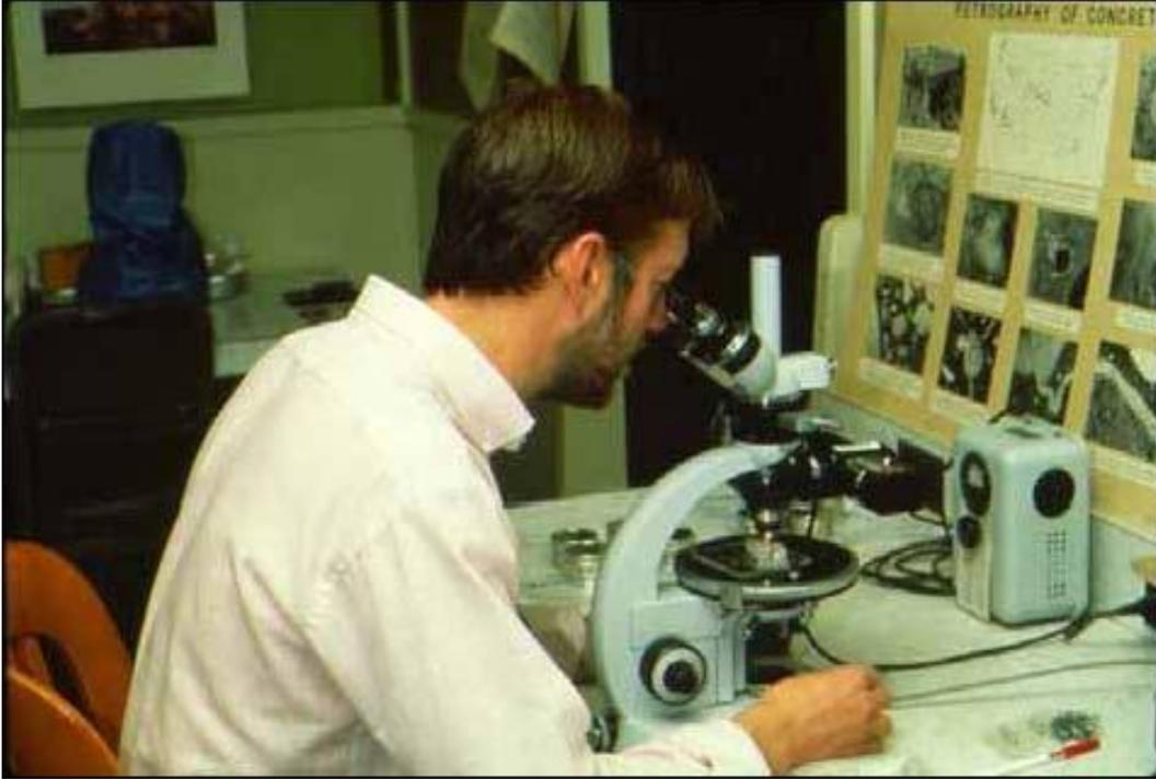
**Figure 4.—Petrographic exam of concrete to help determine cause and extent of damage.**
