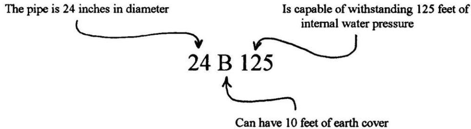
Pipe units usually have various information printed on the inside or outside of the pipe. Other information may be shown on the pipe unit indicating what AWWA or ASTM standard was used to manufacture the pipe. Information on pipe marking required is discussed under pipe types.
