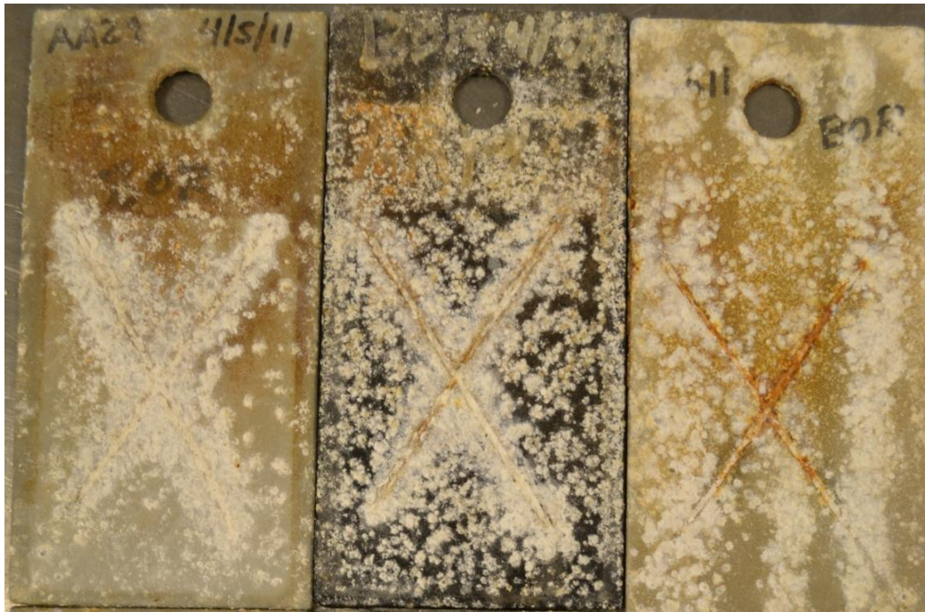
Figure 2.—Effect of thin seal: Aluminum- \text{Al}_2\text{O}_3 systems tested in the BOR corrosion test cycle after 5,040 hours. (a) Amercoat seal, (b) Metco, (c) unsealed.
