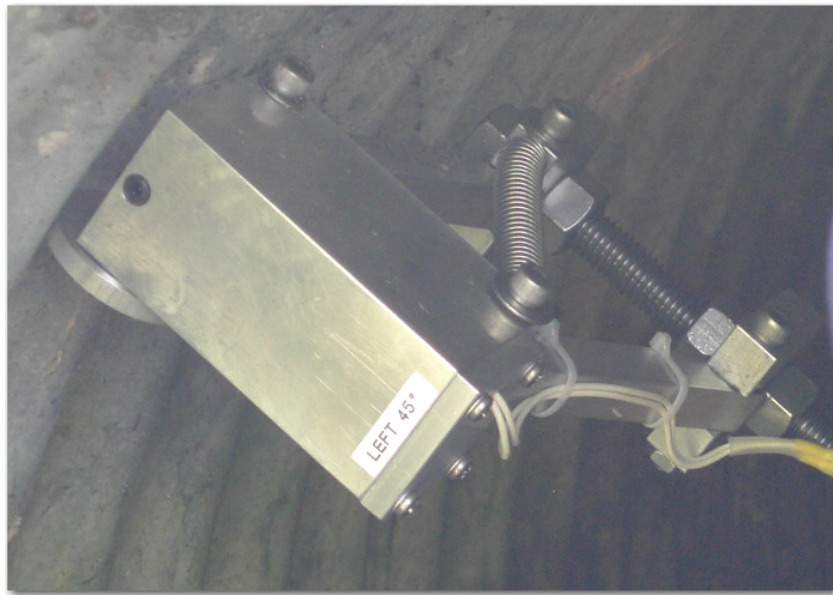
Figure 7.—Revised exciter solenoid assembly with pipe-following wheel.
