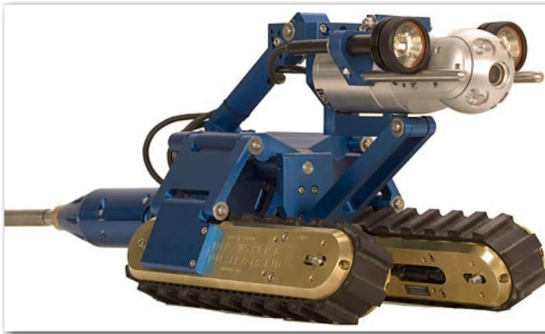
Figure 4.—Pipe crawler with integral video camera and lighting system
