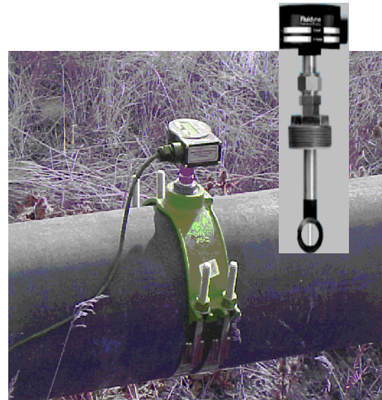
Figure 9.—Fluidyne vortex shedding meter and flow display which is also mounted on a 10-inch pipe. These meters may be used on pipes between 3 and 20 inches in diameter.
