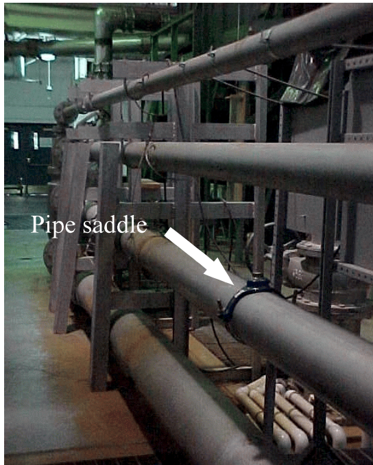
Figure 11.—WRRL pipe test stand showing the pipe saddle on the 8-inch pipe where the flow meters were tested. The pipes in the stand are 4, 6, 8, and 12 inches in diameter.
