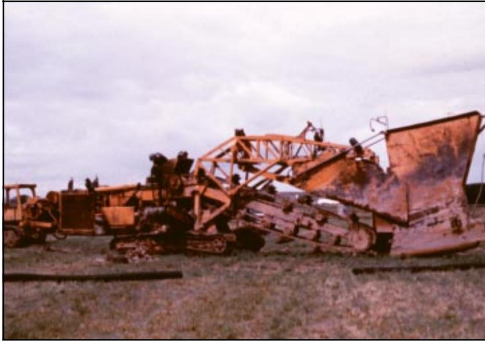
*Figure 8.—Ladder trencher.*
