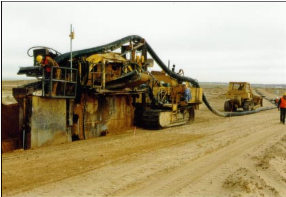
*Figure 7.—Wheel trencher.*
