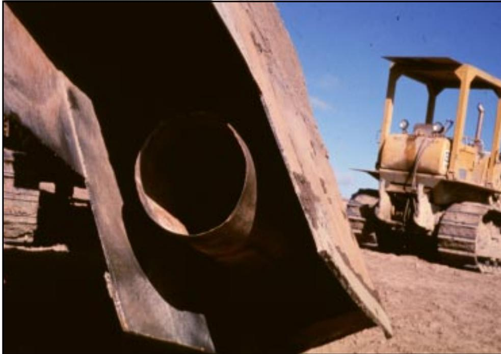
*Figure 10.—Trencher boot arrangement.*
