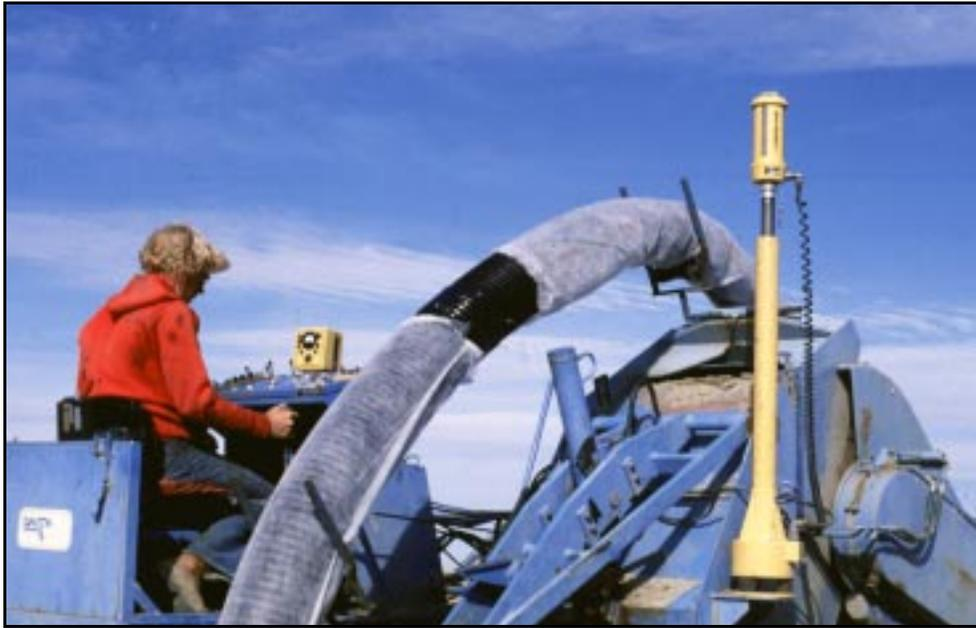
*Figure 3.—Pipe with thin filter sock.*
