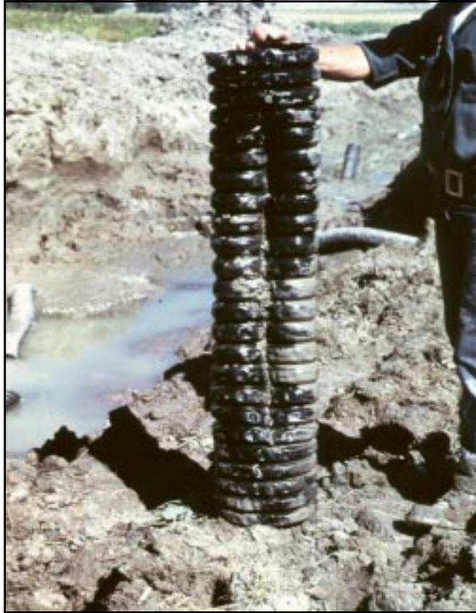
*Figure 1.—Pipe failed due to stretch.*
