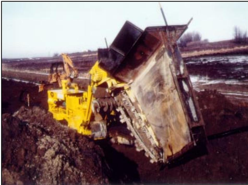
*Figure 9.—Chain trencher.*
