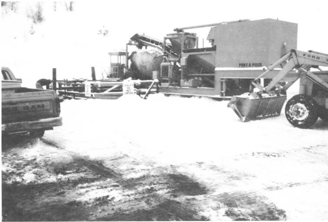
Mobile concrete batch plant operating near the inlet to Blanco Tunnel, a component of the San Juan-Chama diversion system. The plant was designed to the custom specifications of the Chama Field Division.
