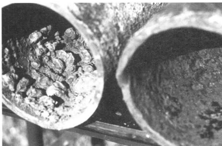
Fifty years of scale accumulation was loosened and dissolved in a day.
