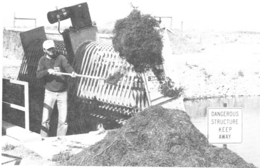
Emil Johnson forks weeds from holding pit. An automated conveyor belt will make this manual task unnecessary in the future.
