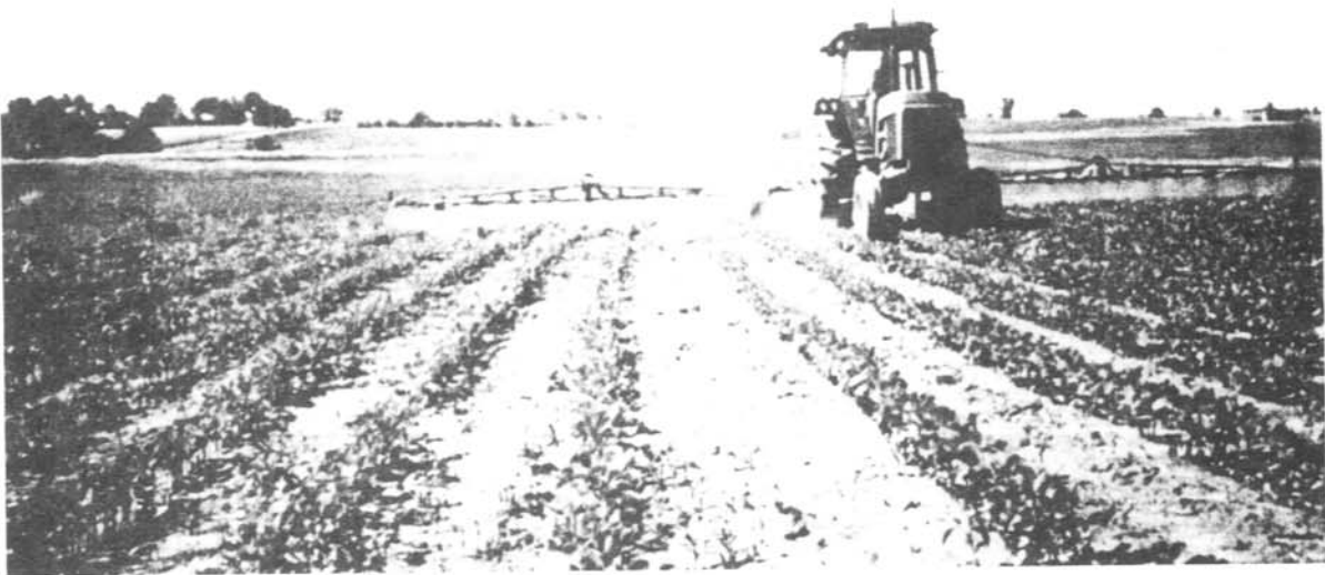
At proper height, the sprayer should provide an even amount of chemical across the full width of the boom
