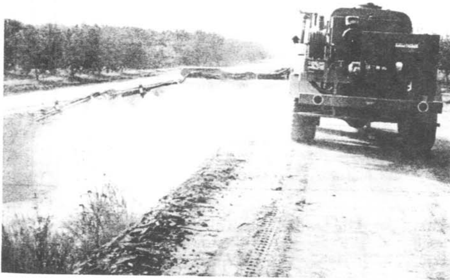
Herbicide application on irrigation ditch with adjustable boom
