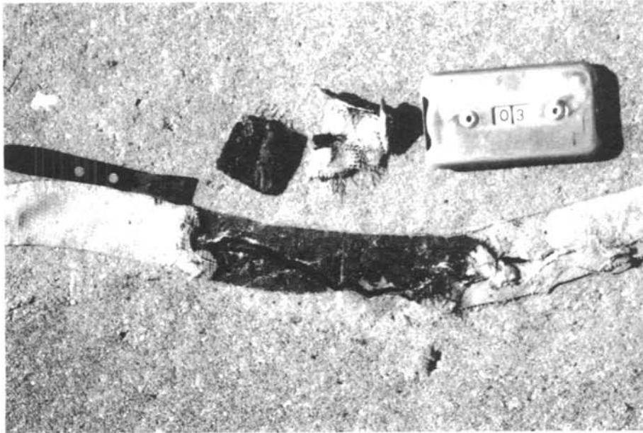
Figure 13. – Reinforced-asphalt mastic tape tends to deteriorate rather quickly, has relatively weak bond, and is difficult to center over wandering cracks.
