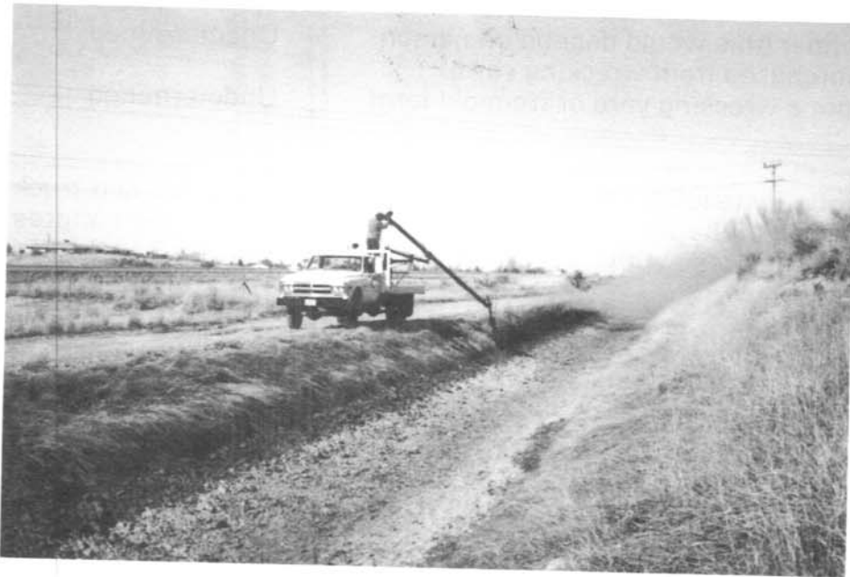
Photo 2. Weedburner mounted on truck and being used in ditch alongside of road.
