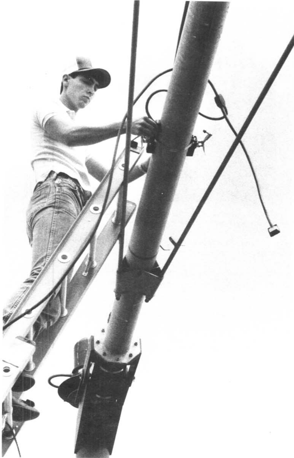
Darrel Evans, Apache, attaches flow-rate measuring equipment in pumping efficiency tests sponsored by OSU and the state Corporation Commission.
