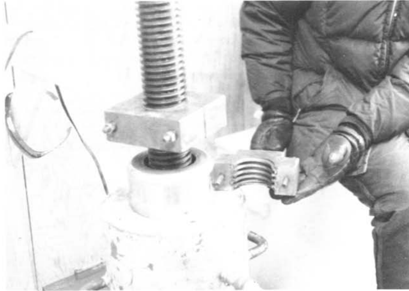
One-half of lower split nut showing threads.
