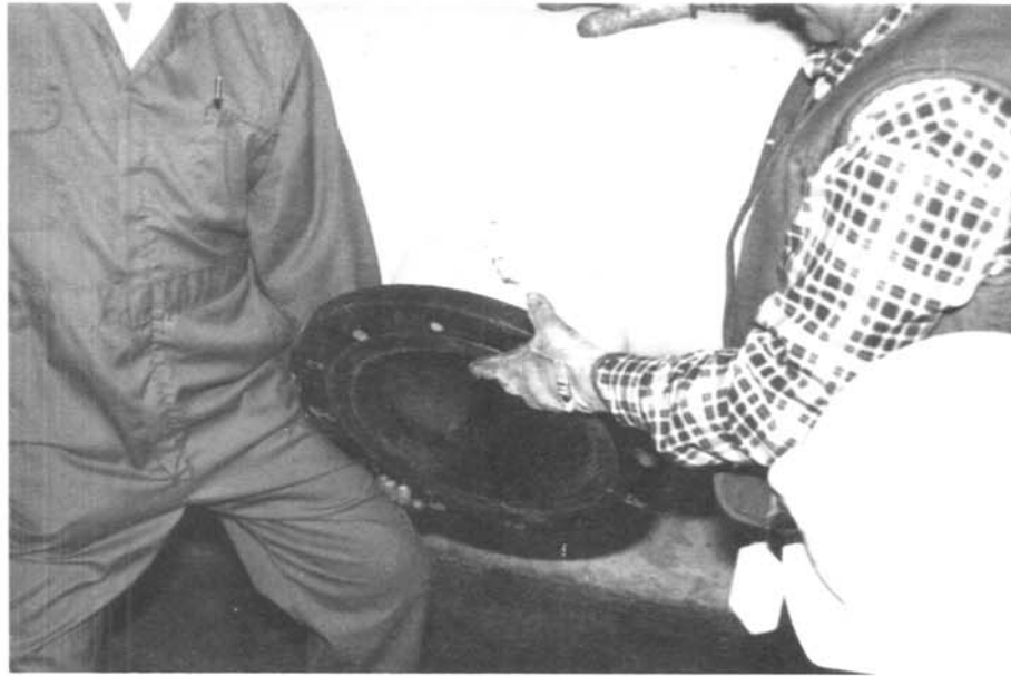
Class E type flange which will replace the sleeve-type couplings.
