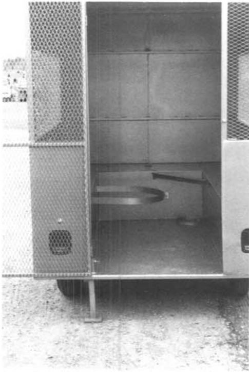
Figure 16.—Trailer has holders for two tanks and a storage bin for dry chemicals.
