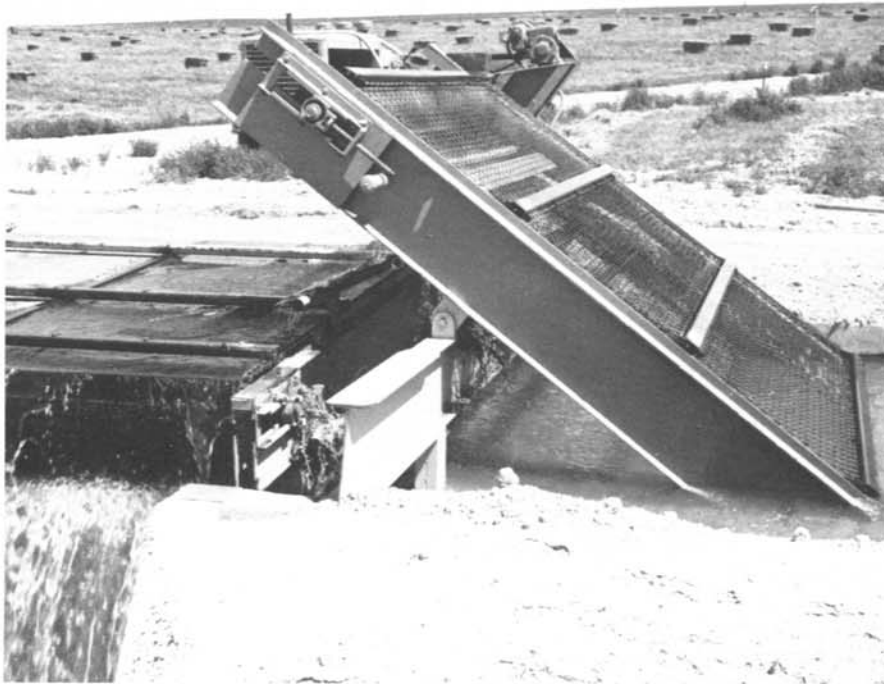
Figure 3.—Side view of canal-type screen. Note the single point pivot mount and the side conveyor.
