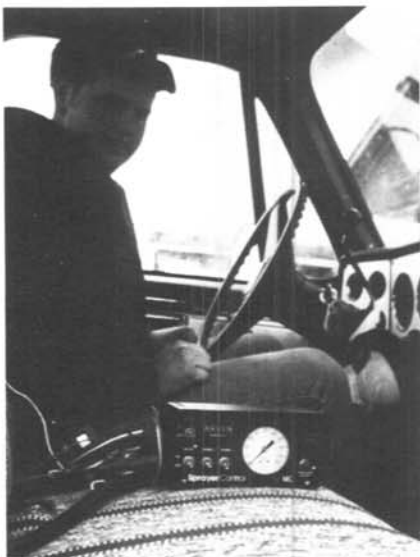
Figure 13.—Remote electrical controls allow Novak to turn the nozzles on and off from the seat of his pickup cab.
