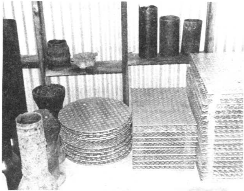
Figure 14.—Metal lids with angle iron welded to bottom to keep them in place.
