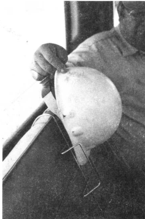
Figure 11.—Hardhat slides easily into holder.
