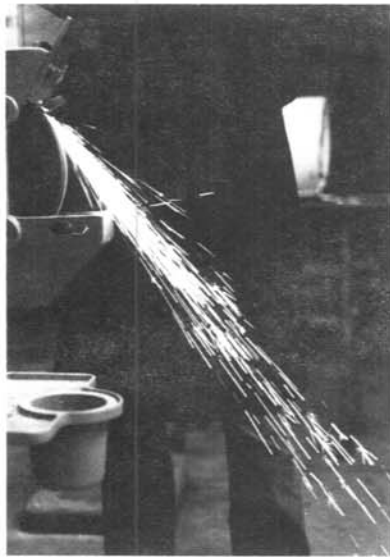
Figure 6.—Low-carbon steel emits long yellowish lines and occasional forks.
