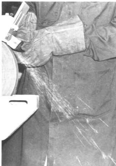
Figure 8.—High-carbon steel emits white lines and bright bursts when ground.
