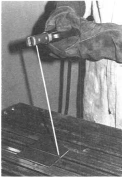
Figure 14.—In flat weld, hold electrode at 15-degree incline angle (in addition of bead).
