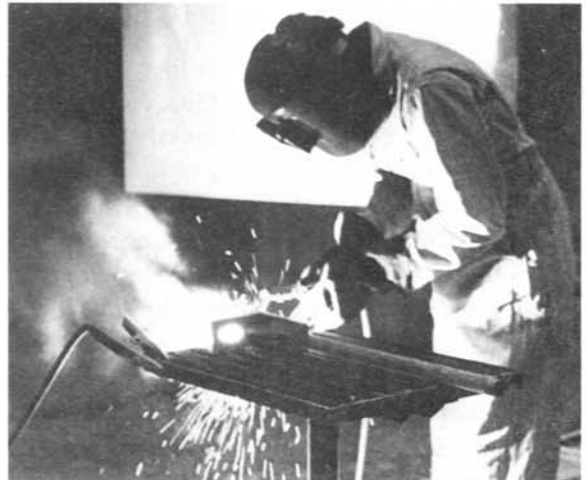
Figure 22.—Set up a fan or some other ventilation system that pulls or blows fumes away from the welding site, as is being done by a portable fan.
