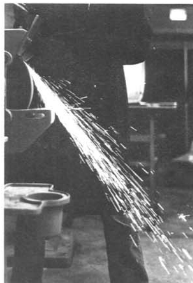
Figure 9.—Malleable cast iron emits somewhat reddish carrier lines, when ground.
