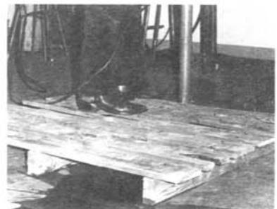
Figure 24.—Wooden pallet can give welder a dry place to stand, when area is wet.
