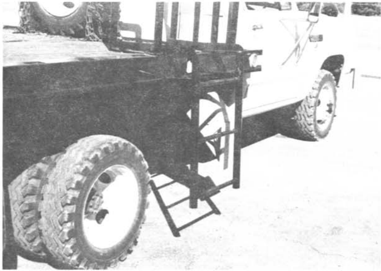
Figure 4.—Ladder in the lowered position. The distance between the top rung and the truck bed allows ample room for safe footing.
