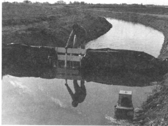
Figure 6.—Bulkhead/weir No. 2—Head being checked by Mr. Colianni and will be correlated to water stage recorder.
