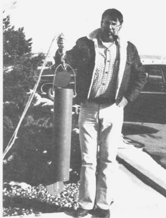
Figure 16. A. W. Kinsey is holding sawdust dispenser with both flap doors open, as it would appear while releasing the sealant material.
