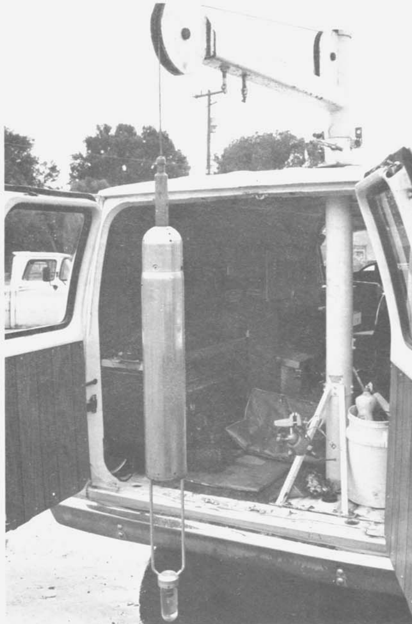
Figure 14. Once the van is backed up to a well, camera and light (located in front of lens tube) are lowered with this L-boom and winch.
