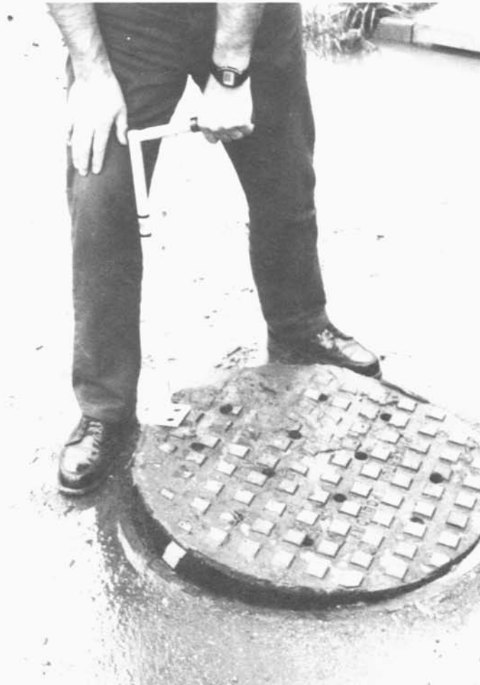
Figure 10.-The hook is inserted into the manhole lifting hole or ring. The hook is tight against the inside of the lid and lifts the lid off with ease.
