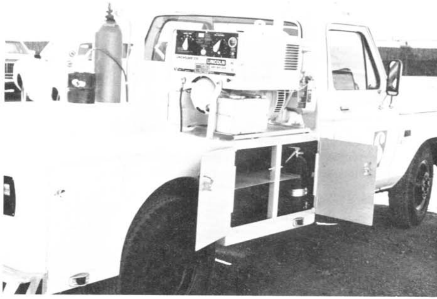
Figure 10.—Back view of arc welder and compartment with fire extinguisher.
