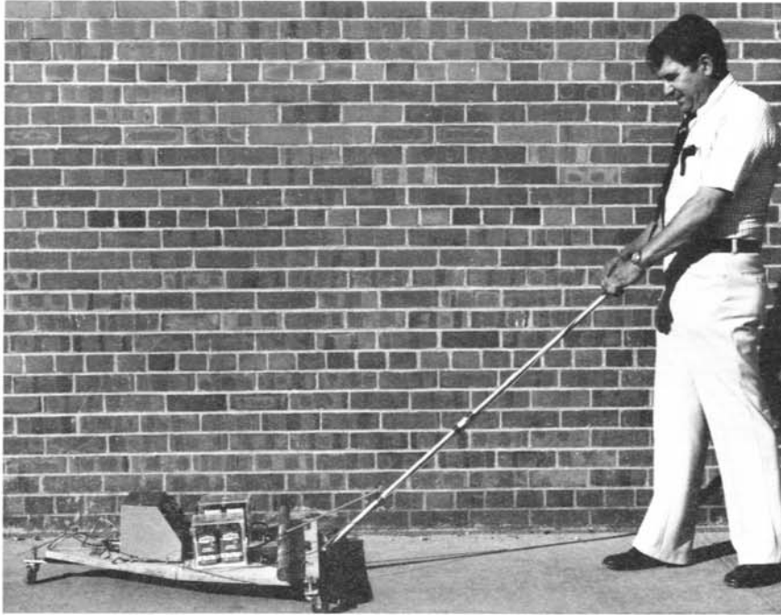
Figure 1.—The prototype electronic void detector is demonstrated by Manuel Guitierrez. Although still in the experimental stage, the device has been successfully tested.
