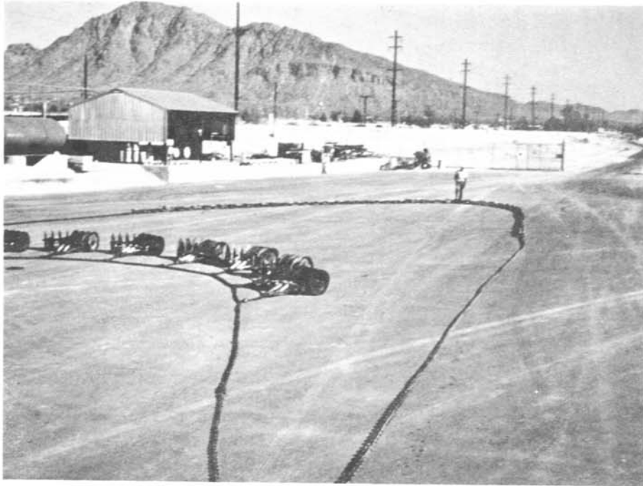
Figure 11. Disc and anchor chain shown in dragging arrangement at Northside Construction and Maintenance Headquarters. Photo PX-D-60887.
