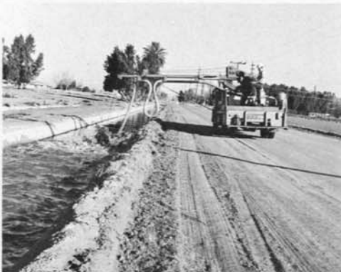
COVER PHOTOGRAPH: This is a turbine compressor and it is shown operating in a lined channel using a contoured nozzle, as described in this Bulletin. Photo PX-D-60882
