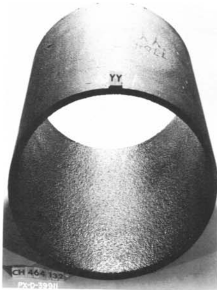
Fig. 2A. Pipe "YY" before testing. Three coats of coal-tar paint, CA-50, second coat reinforced with ASTM C-190 Ottawa sand.
