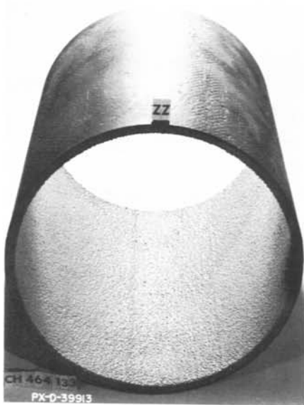
Fig. 2C. Pipe "ZZ" before testing. Lining consists of four coats of red-lead priming paint, TT-P-86a, Type IV, second coat reinforced with No. 20-30 mesh Ottawa sand (ASTM C-190).
