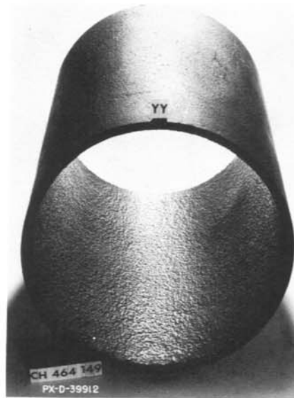
Fig. 2B. Pipe "YY" after testing. The only visible damage is the removal of the CA-50 from the tops of sand grains. View shows condition after four runs.
