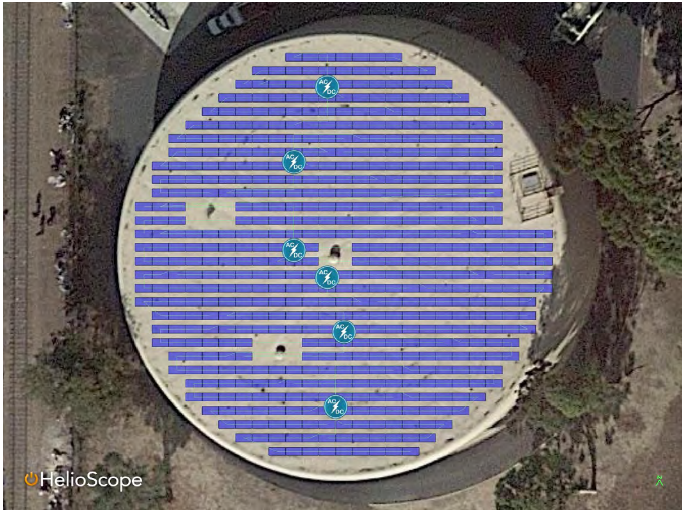
East – This array utilizes the roof space of the single storage tank, while taking into account existing equipment that limits the available space for the installation of solar PV modules. This array would likely utilize a ballast mounted system, pending an in-depth structural analysis.
