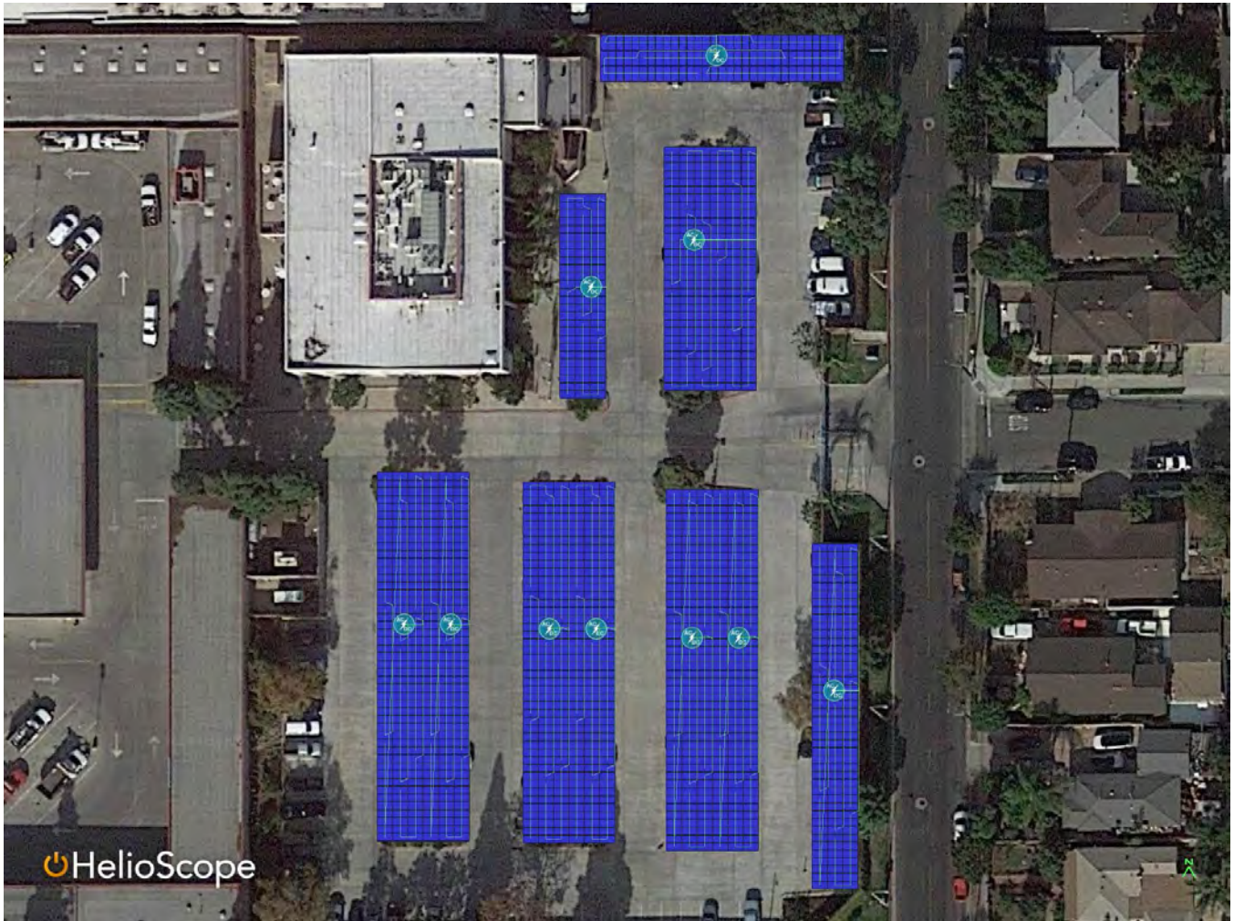
City Yard Caption – This array utilizes available parking lot space using solar carport structures. It is assumed that any trees causing shading will be removed by the city to increase the available space. Since this array would utilize a series of carport structures, a soils analysis will be required.
