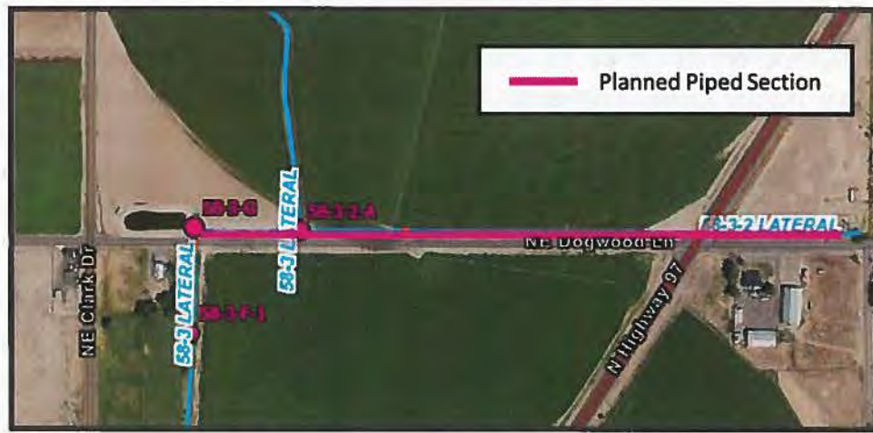
Figure 3. Lateral 58-3-2 Piping Project. Shown in pink is the 1,900 ft stretch of canal to be replaced by buried pipe. This project parallels Dogwood Ln and cuts under Hwy 97.
