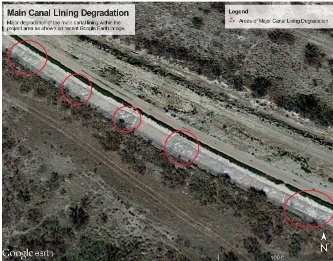
Photo 2: Main canal deterioration as shown in a Google Earth image. Note: 5 degraded areas over 300ft.
