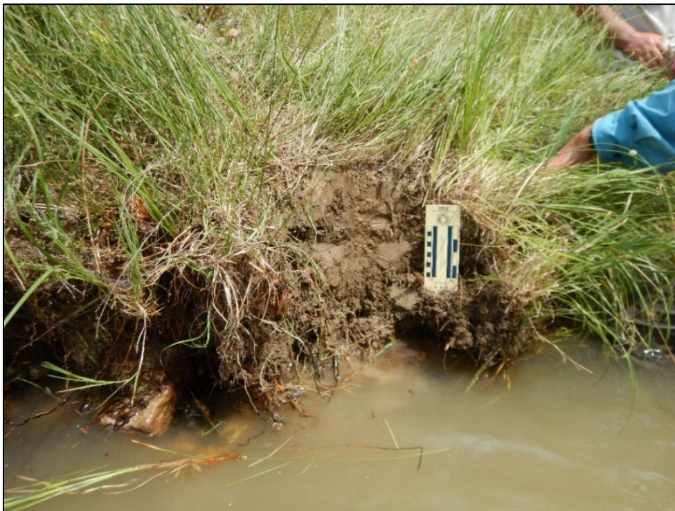
Figure 9. Root reinforcement of the channel bank by Palustrine Emergent Wetland vegetation, including sedges and rushes (RM 15) (RCFP) (Harvey 2022 Section 3.3.1. Floodplain and Aquatic Vegetation ).
