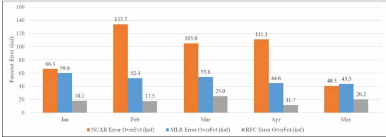
Figure 19. Average monthly over-forecasted errors for the NCAR, MLR, and NWRFC hindcast methods
