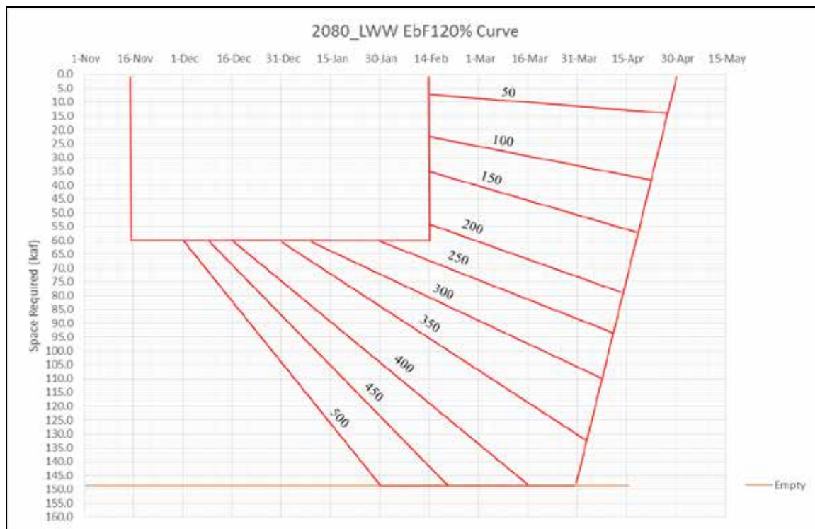
Figure 42. EbF120% curve developed using the 2080 LWW scenario dataset and 2,000 cfs maximum flood discharge target
