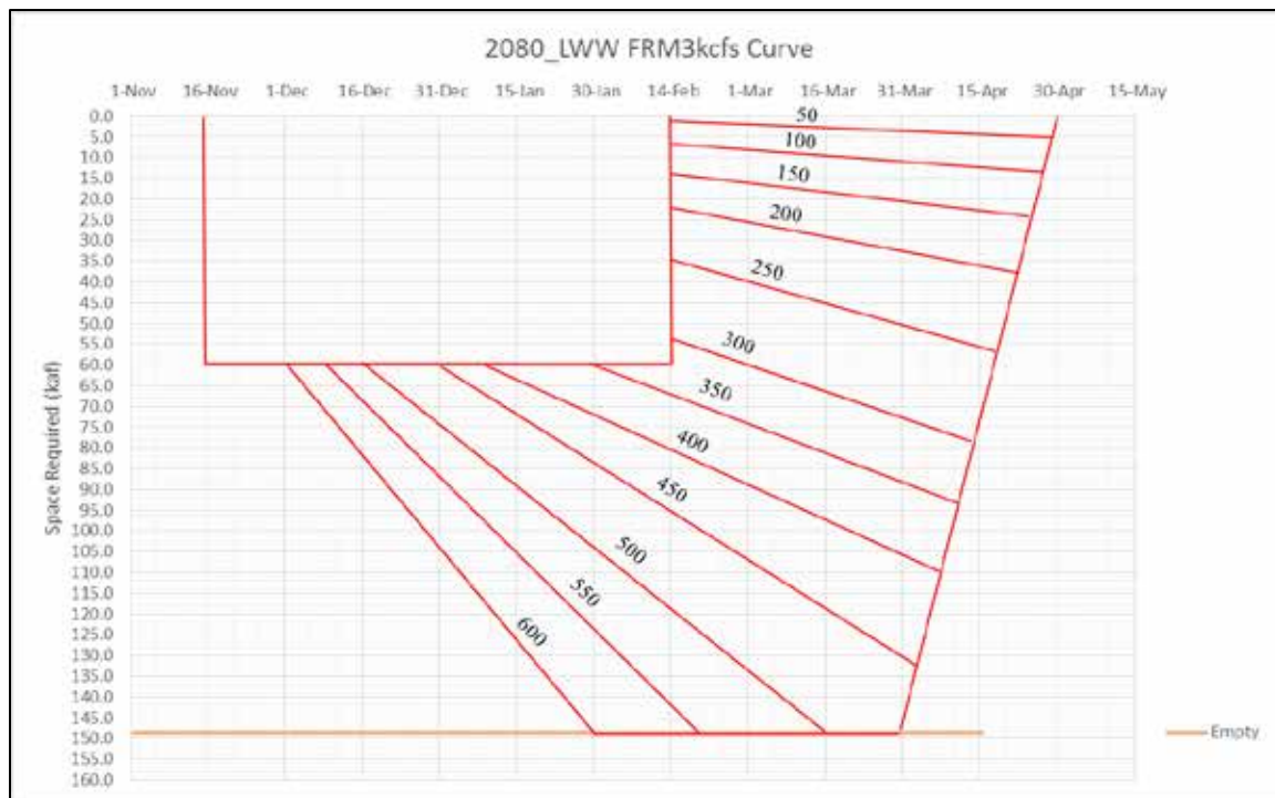
Figure 41. FRM3kcfs curve developed using the 2080 LWW scenario dataset and 3,000 cfs maximum flood discharge target
