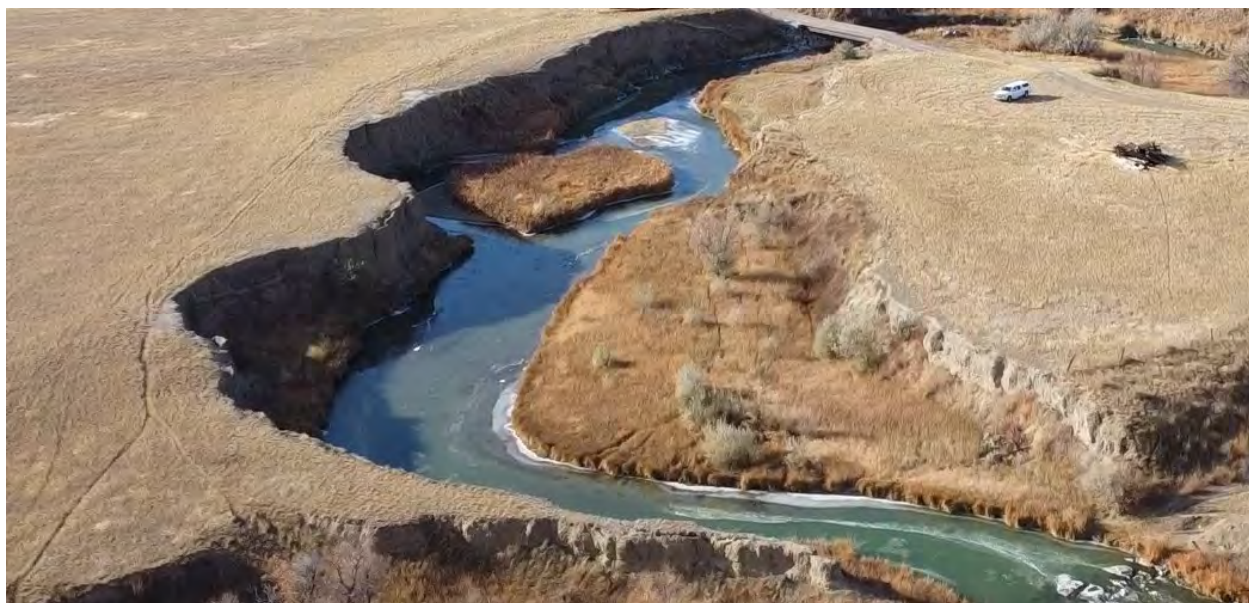
Photo 6, November 2, 2021. View upstream showing steep channel margins on passive edge and island; preliminary hydraulic modeling shows little hydrologic connectivity between these surfaces and the creek.
