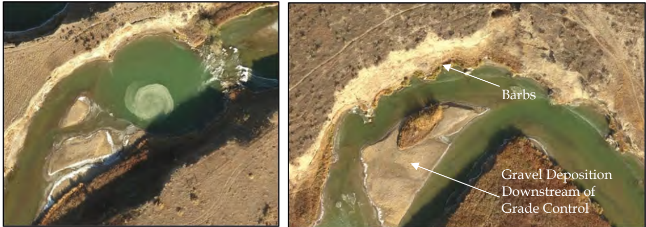
Photo 3, November 2, 2021. Existing Grade Control Structure (left) and Photo 4, November 2, 2021. Barb Series (right)
