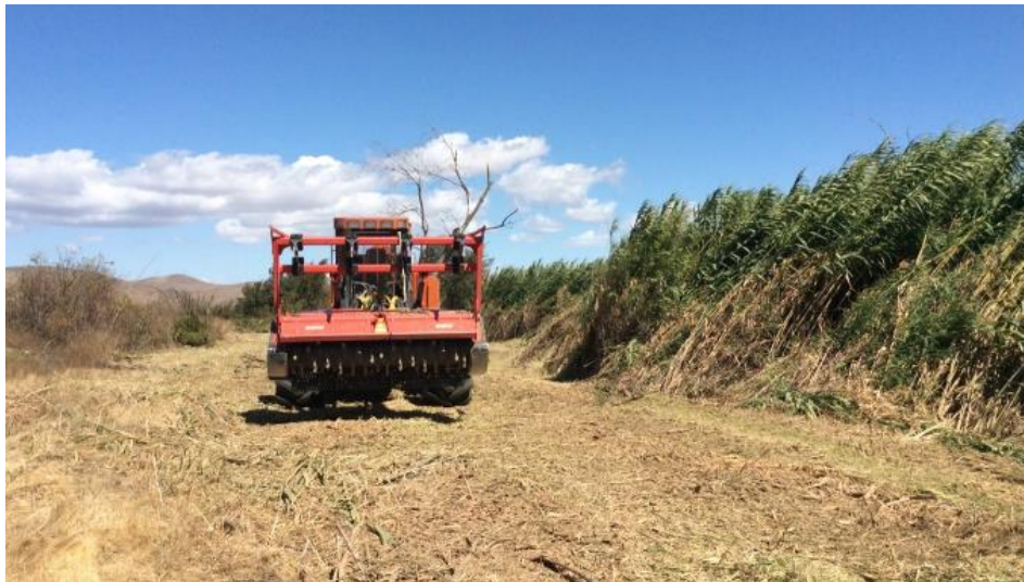
Figure 4. Mowers masticate arundo to a layer of mulch in the first year of work
