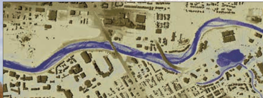
Confined River Channel - the channel in this reach exhibits confinement, poor channel form, lack of complexity and straightening.
