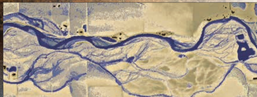
Complex River Channel - the channel in this reach exhibits complexity, sinuosity and connected floodplain. Blue areas are low below the water surface in high flow conditions. Brown areas are well above the water surface.
