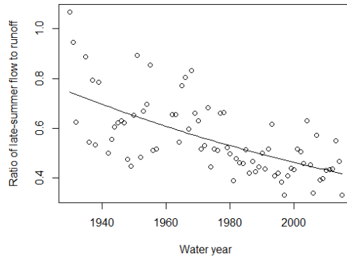
Ratio of late-summer (August 1 – September 30) mean flow in the Teton River to mean flow during runoff (May 15 – July 15). Curve depicts statistically significant decline in this base-to-peak flow ratio over time.
