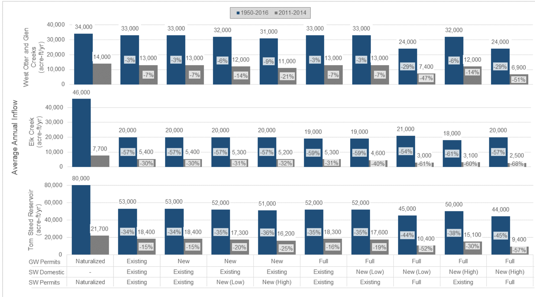
Figure 23. Average annual inflows into Tom Steed Reservoir under a range of groundwater and stream-water use scenarios over the period of record (1950-2016) and during the drought of record (2011-2014).
