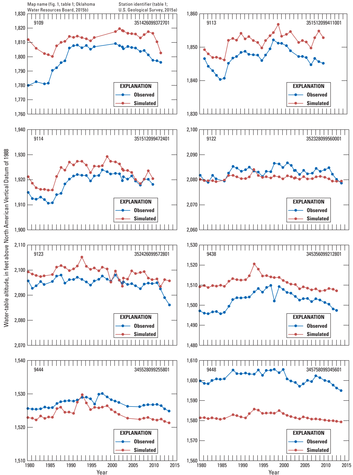
Figure 28. Observed and simulated water-table altitudes for the numerical groundwater-flow model of the North Fork Red River aquifer, 1980–2013.—Continued
